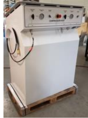
Figure 7. MTA Boost Compressor Fueling Post.
