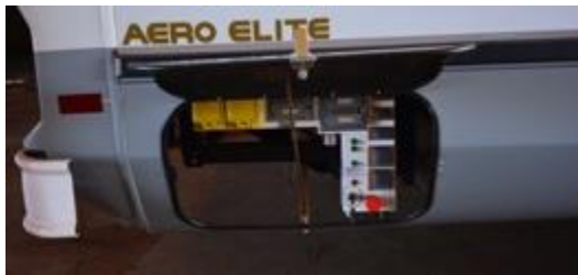
Figure 9. Bus Export Power Unit.
