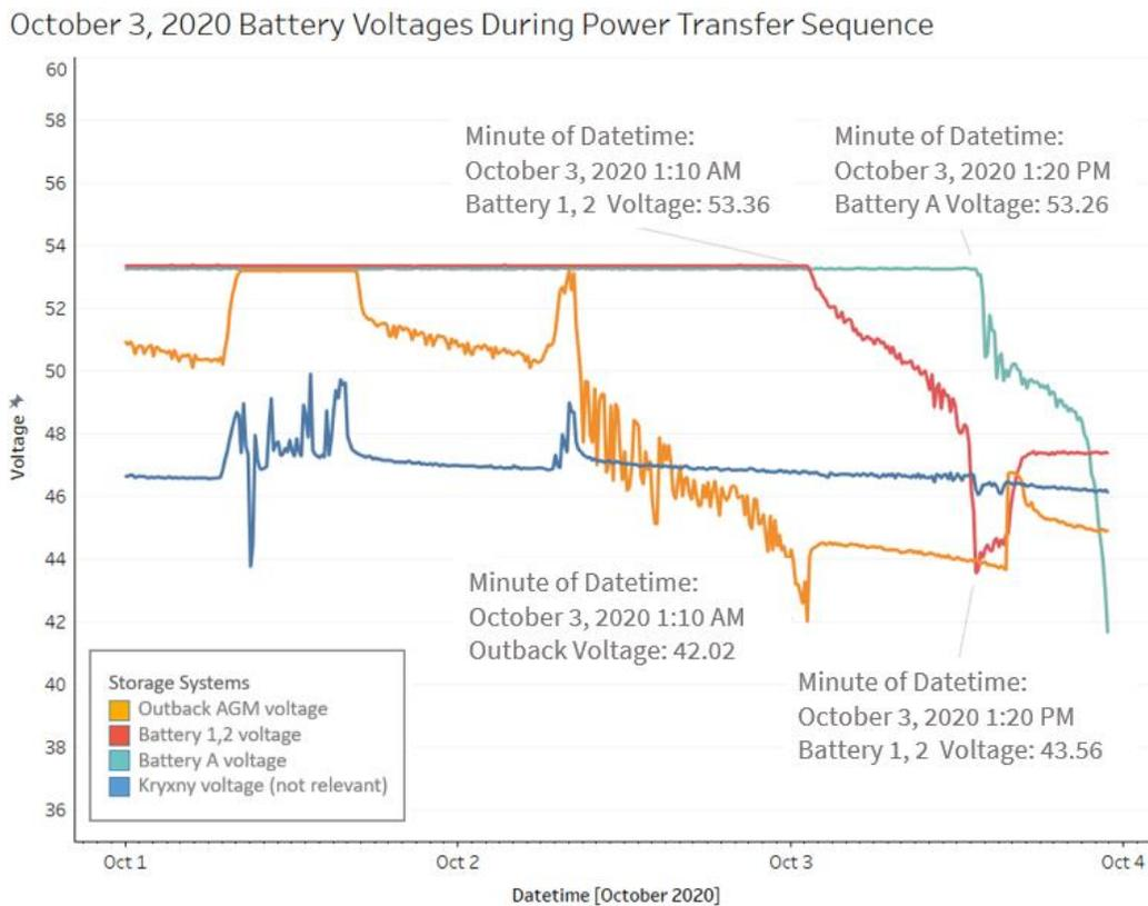
Figure 9. Transfer of load from primary to backup storage systems based on battery voltage (“Battery 1, 2” refers to the Sungold/1,2 system and “Battery A” refers to the Xijia/A system).
