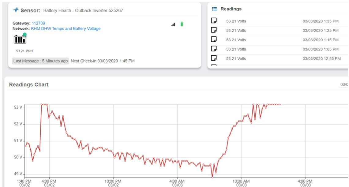
Figure 4. Overnight losses for Outback inverter, includes baseload and standby losses.
