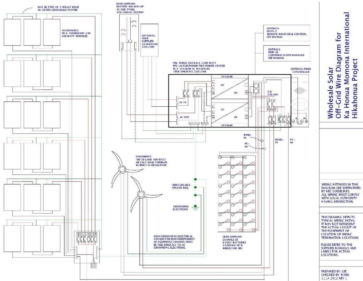
Figure 3. Original KHM renewable energy system design schematic.
