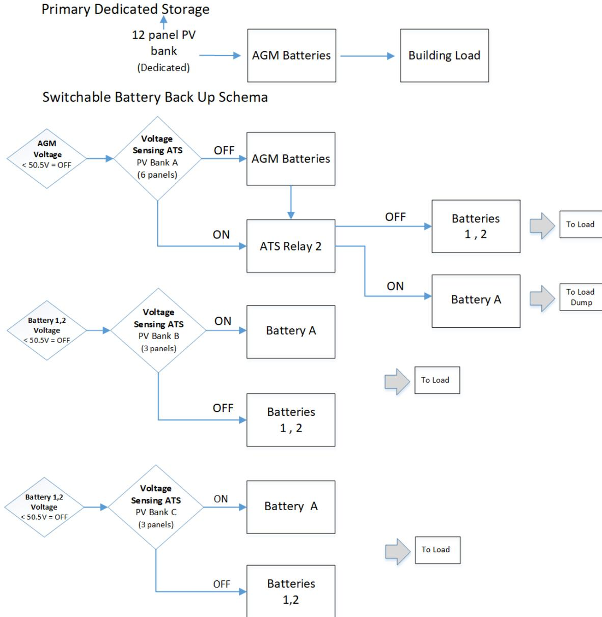
Notes: PV banks A, B, C all assignable to backup banks 1,2 or A, depending on the state of charge of primary and backup. B and C banks can be manually assigned via web app to either storage, e.g., 3 to one, and 3 to the other, or 6 to either. The load dump circuit is dedicated to Bank A, and will only operate when primary and secondary remain above 50.5V.
