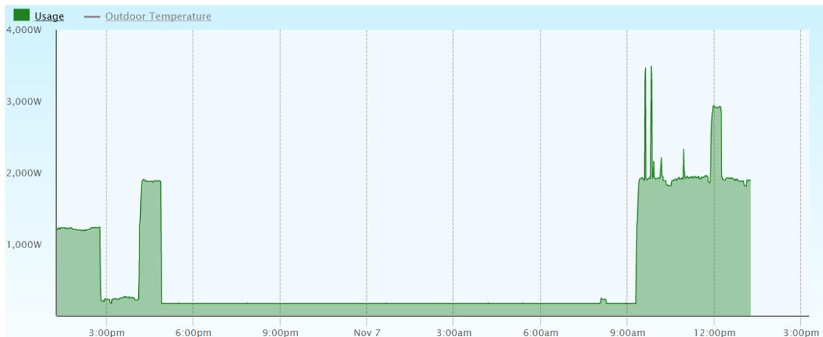
Figure 2. 24-hour load profile with varying load conditions: baseload (250 W), typical (2,000 W) and short peaks (2,700-3,000 W).
