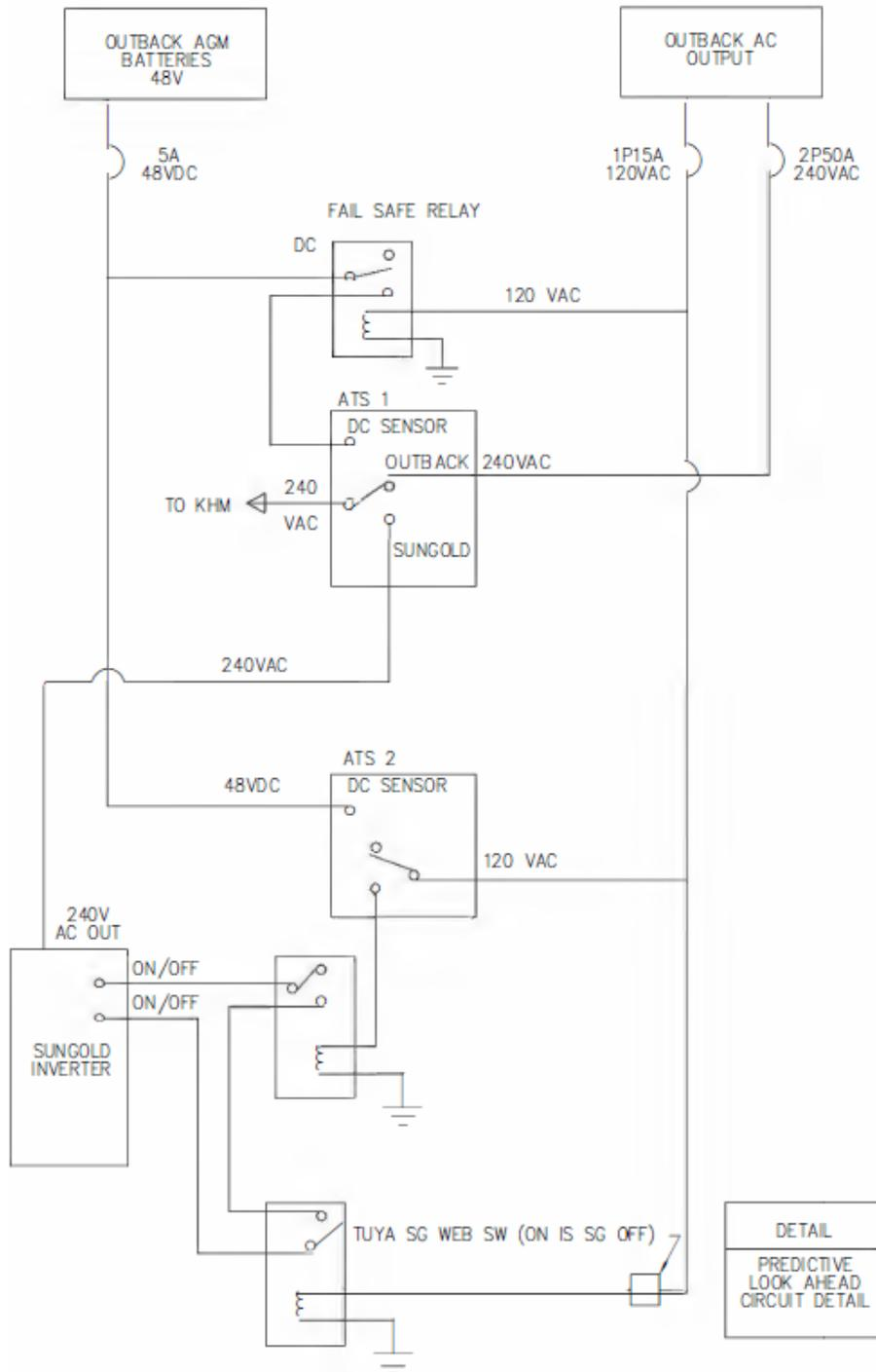
Figure 7. Switching schematic for Predictive Look Ahead Programming.
