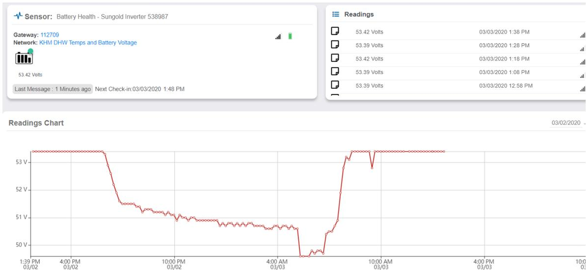
Figure 5. Overnight losses for Sungold inverter, includes no-load standby losses only.
