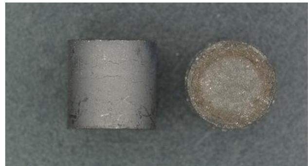
Figure 1. Biocarbon pellets produced from TPP biochar.
