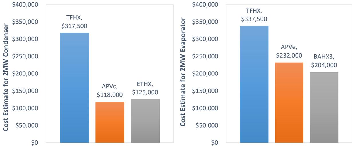
*Figure 14. Comparison of estimated cost for 2MW heat exchanger.*
