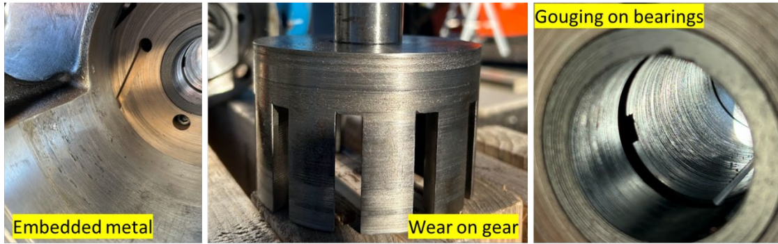
Figure 7. Recirc pump damage.
