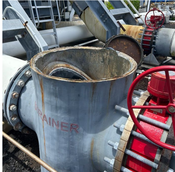
Figure 14. Top part of the strainer sheared off.
