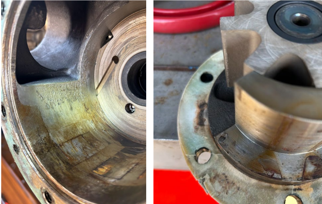
Figure 9. Metal chunks embedded in the pump casing (left) and pump head (right).
