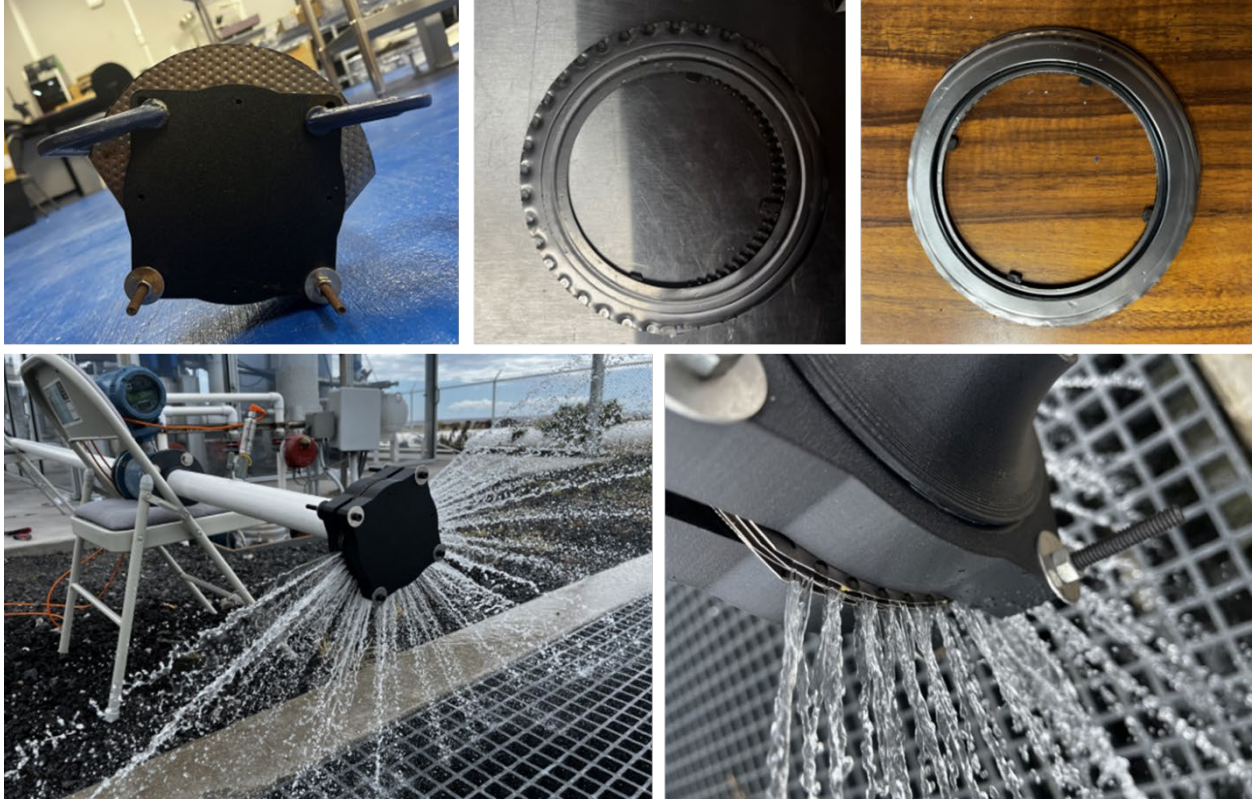
Figure 10. (top, left to right). Plates were cut such that flow passed through the (top left) manifold insert + transition + 1" pattern, (top middle) manifold insert + transition zone, and (top right) manifold insert only.
