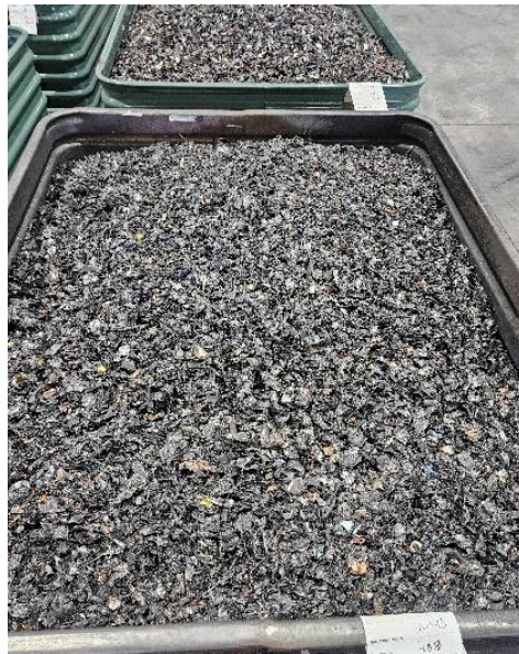
Figure 23. Output from crude shred of lithium-ion batteries 167 .
