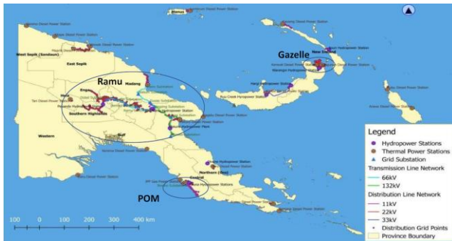
Figure 1. PPL's main power systems in PNG.
