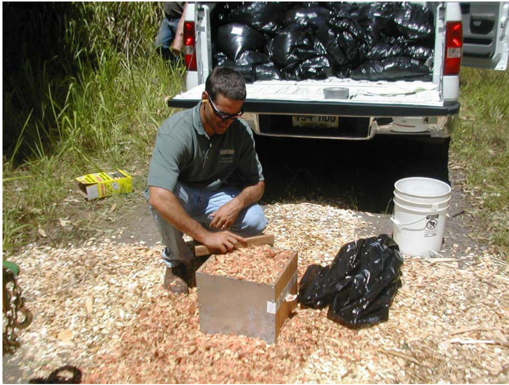
Figure 3. Measurement of bulk density according to ASTM 873 [3].
