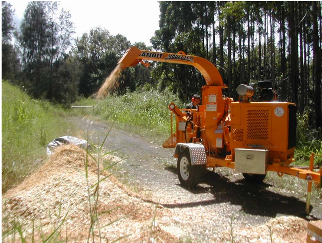
Figure 2. Badger Model 150 chipper used to reduce bolts to chips for sampling.
