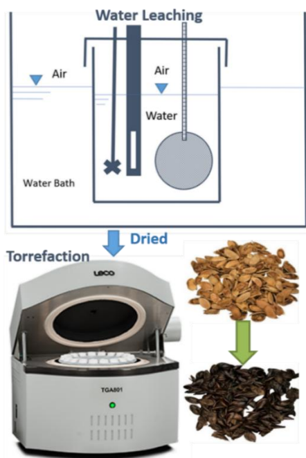
Figure 22. Laboratory scale leaching and torrefaction test equipment.
