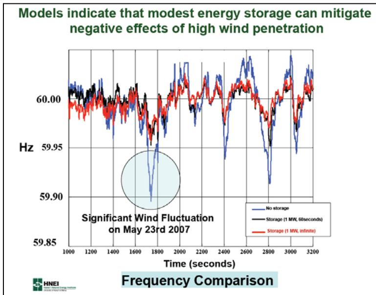
**Figure 1: Effect of Energy Storage on Grid Frequency Regulation**
