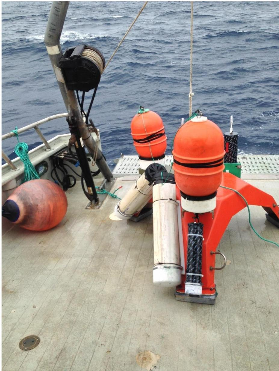
Figure 1 Sea Spider prior to deployment with the larger rope canisters for deployment at the 60m site.
