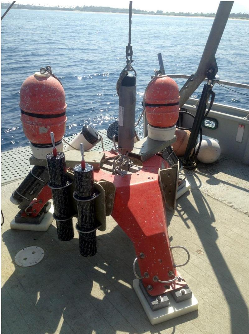
Figure 3 UH Sea Spider Hydrophone before Deployment
