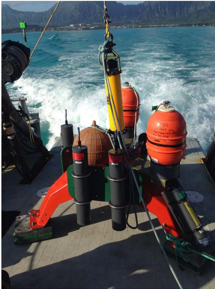
Figure 1 UW Sea Spider, Acoustic Release, and Winch
