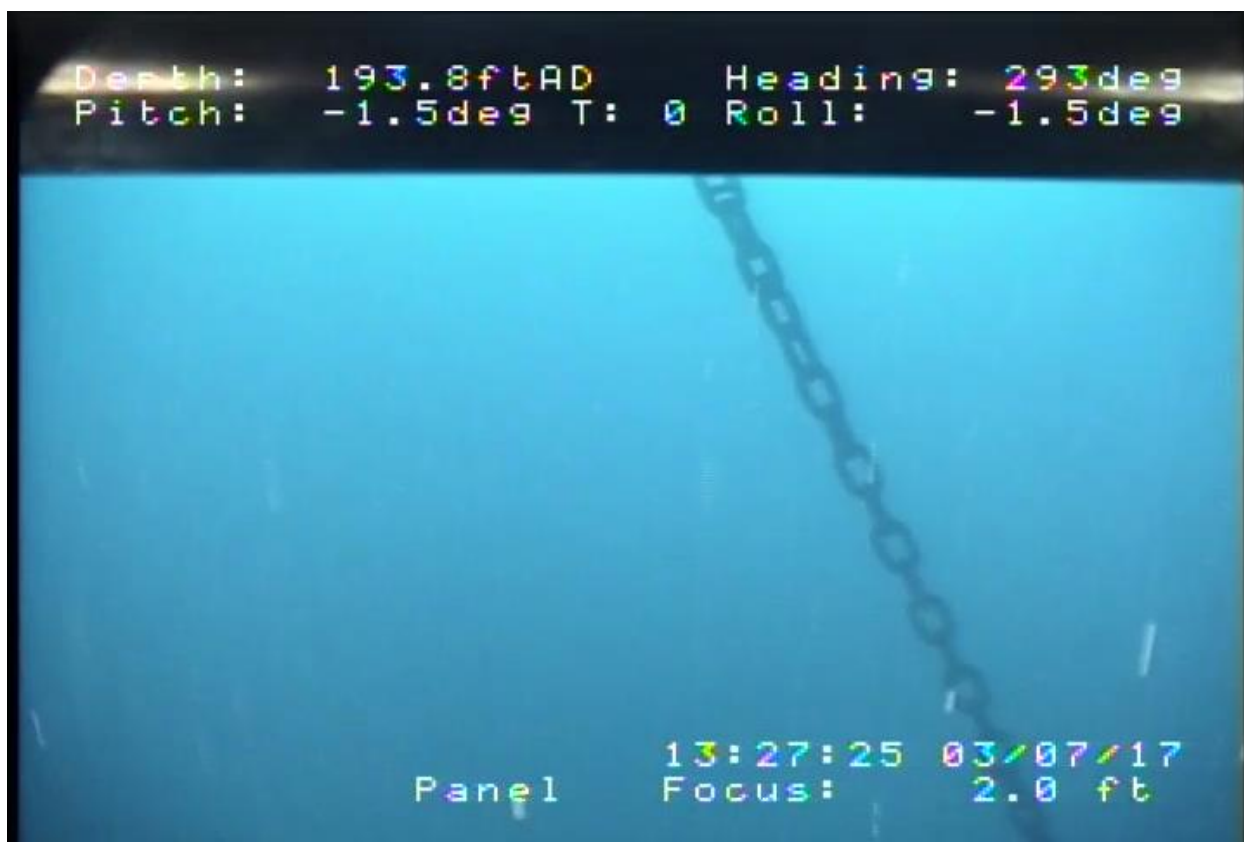
Figure 4-14 A2-ML-4 Missing Studs
