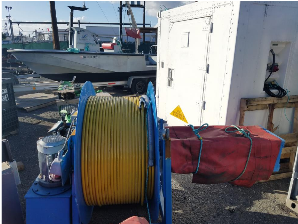
Figure 5. Deck Winch with Super Mohawk ROV Umbilical Loaded onto Winch
