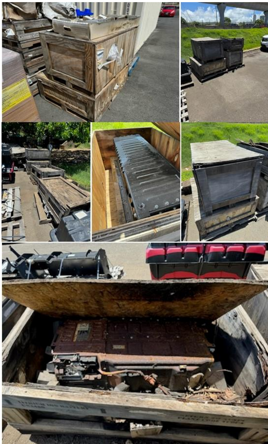
Figure 8. Images of improperly stockpiled LIBs at commercial business.
