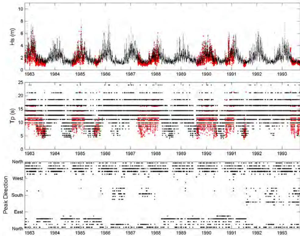
Figure 56- Comparison of recorded (red) and hindcast (black) wave parameters at the Barking Sands buoy.
