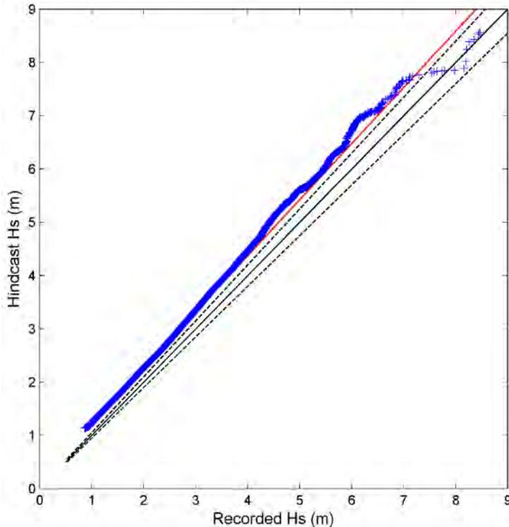
Figure 35- Quantile-quantile plot of recorded and hindcast significant wave heights at buoy #51101. Blue crosses represent data pair at 0.002 percentile increment, black line denotes perfect match, black dash lines delineate the  $\pm 5\%$  error bounds, and red line is the linear regression.
