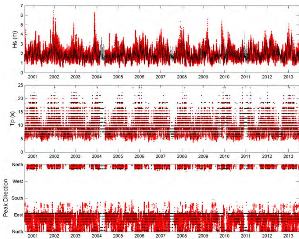
Figure 46- Comparison of recorded (red) and hindcast (black) wave parameters at the Mokapu buoy.
