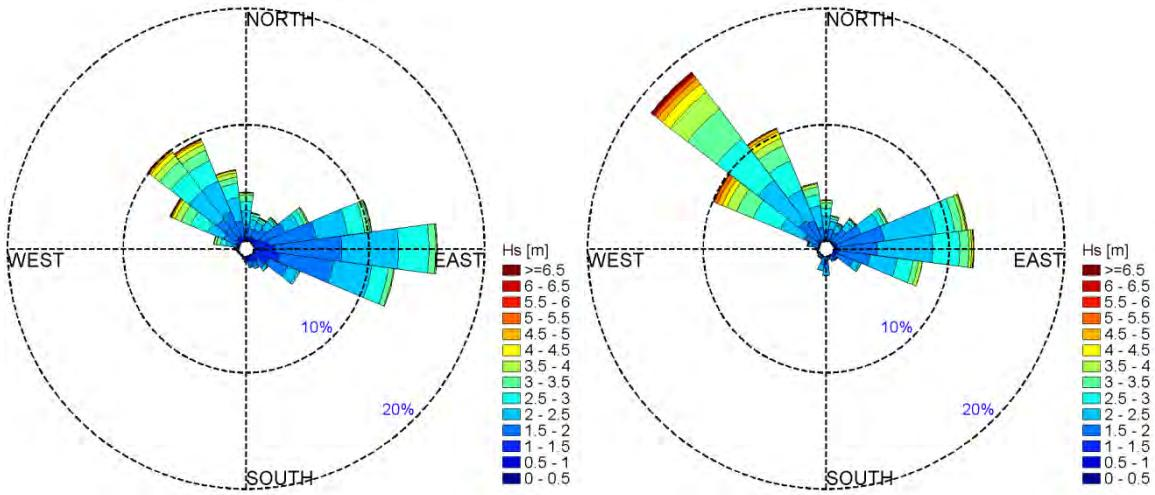
Figure 40- Rose plots of recorded (left) and hindcast (right) significant wave heights at buoy #51100.
