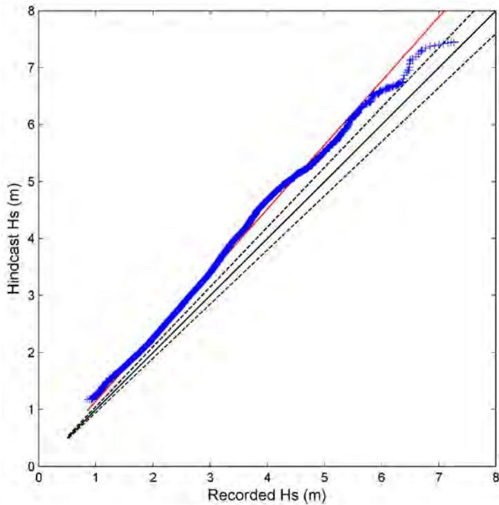
Figure 34- Quantile-quantile plot of recorded and hindcast significant wave heights at buoy #51100. Blue crosses represent data pair at 0.002 percentile increment, black line denotes perfect match, black dash lines delineate the  $\pm 5\%$  error bounds, and red line is the linear regression.
