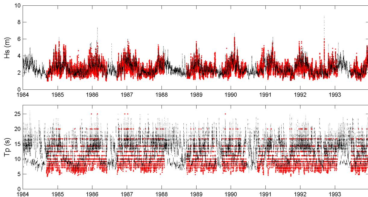
Figure 16- Comparison of recorded (red) and hindcast (black) wave parameters at buoy #51002 from 1984 to 1993.
