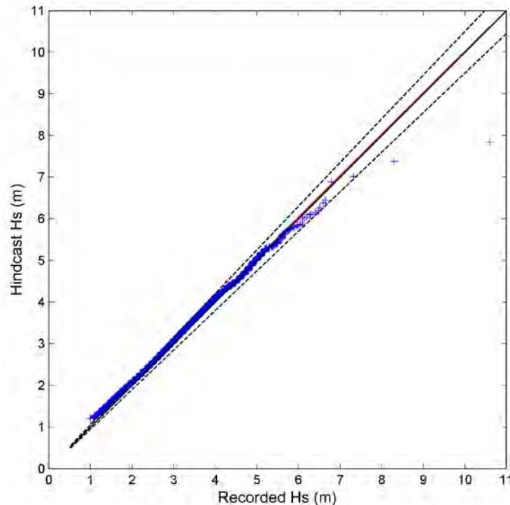
Figure 33- Quantile-quantile plot of recorded and hindcast significant wave heights at buoy #51004. Blue crosses represent data pair at 0.002 percentile increment, black line denotes perfect match, black dash lines delineate the  $\pm 5\%$  error bounds, and red line is the linear regression.
