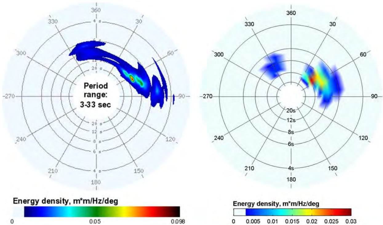
Figure 82- Two-dimensional spectra estimated from WETS Waverider records (left) and hindcast model (right) at 4:00 PM May 5, 2013.
