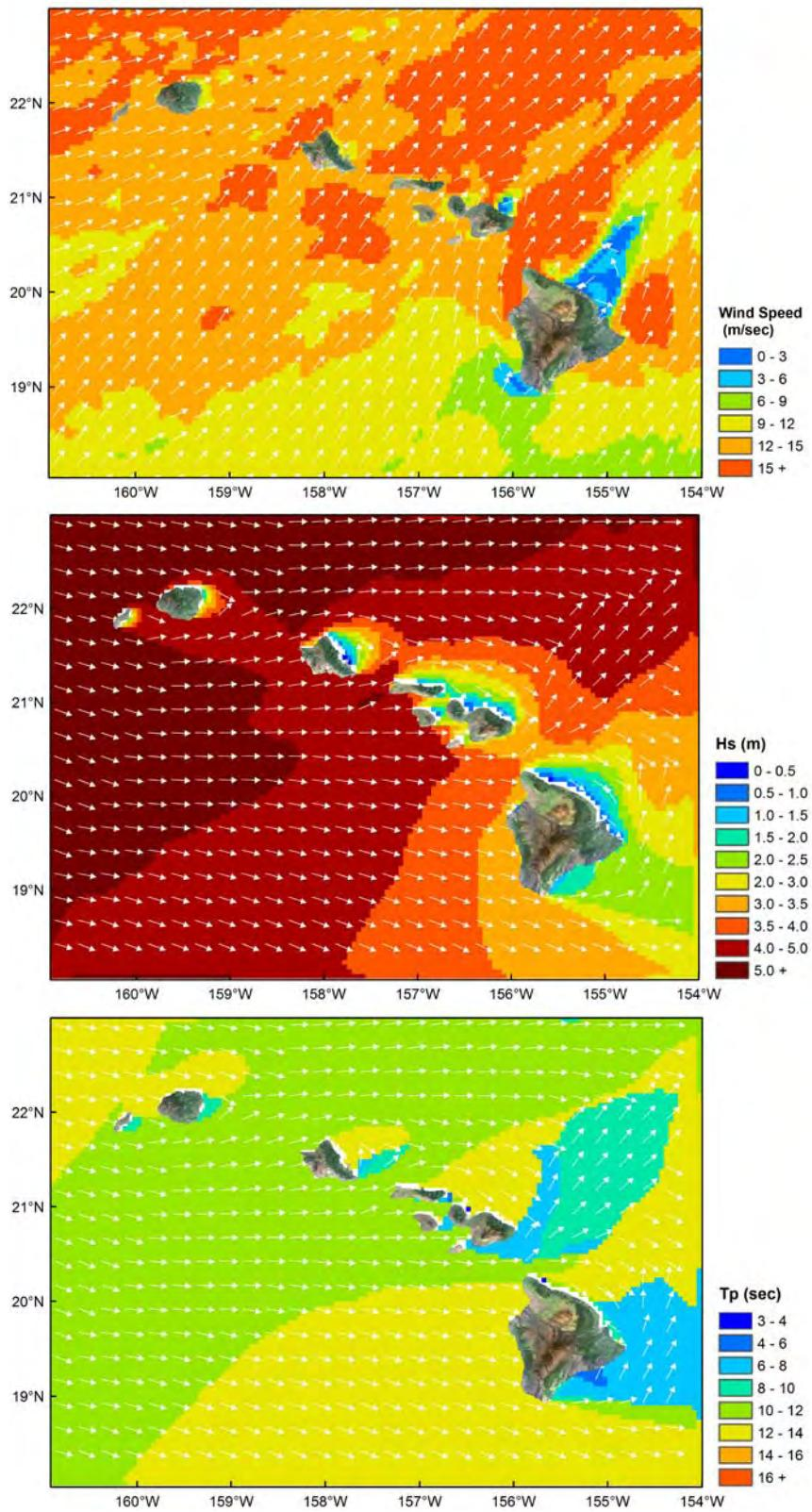
Figure 9- Wind velocity, significant wave height, and peak period during a Kona storm at 9:00 AM January 11, 1980UTC.
