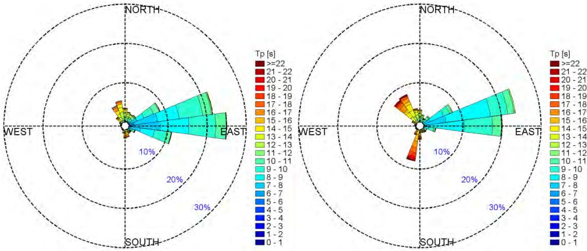
Figure 39- Rose plots of recorded (left) and hindcast (right) peak periods at buoy #51004.
