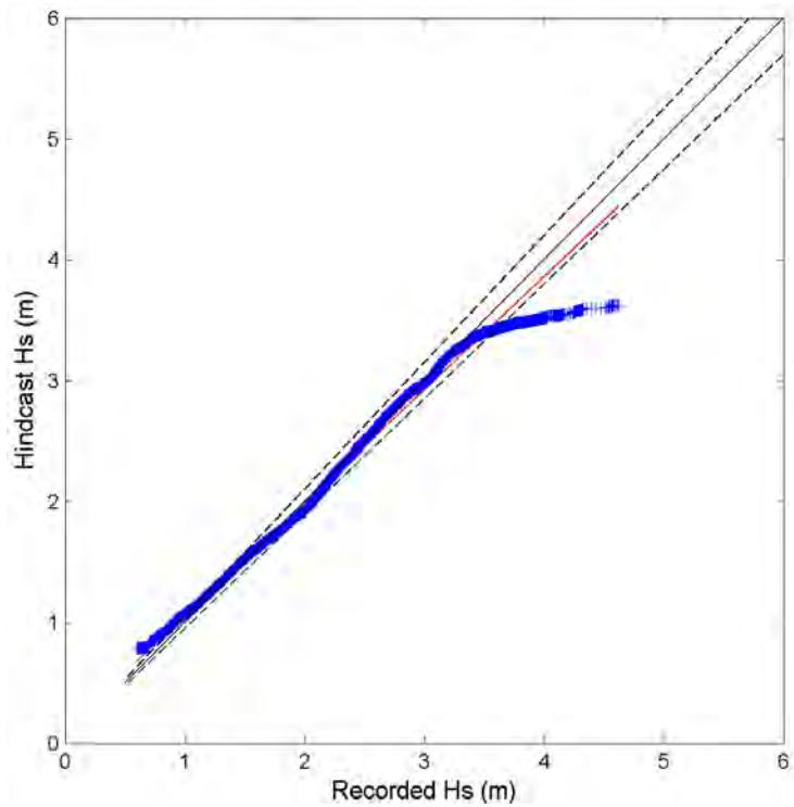
Figure 67- Quantile-quantile plot of recorded and hindcast significant wave heights at the Hilo buoy. Blue crosses represent data pair at 0.002 percentile increment, black line denotes perfect match, black dash lines delineate the  $\pm 5\%$  error bounds, and red line is the linear regression.
