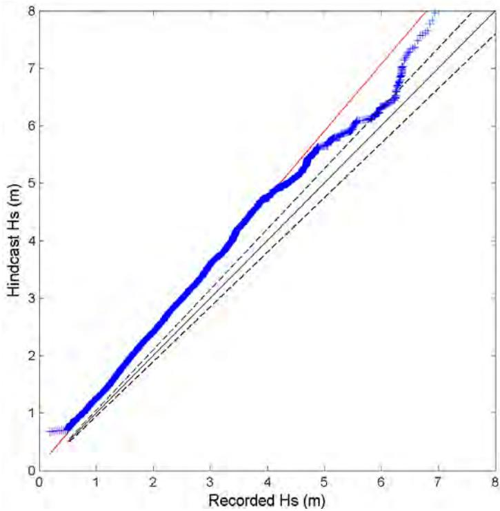
Figure 64- Quantile-quantile plot of recorded and hindcast significant wave heights at the Barking Sands buoy. Blue crosses represent data pair at 0.002 percentile increment, black line denotes perfect match, black dash lines delineate the  $\pm 5\%$  error bounds, and red line is the linear regression.
