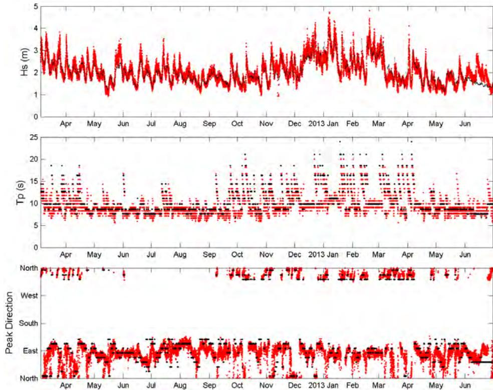
Figure 59- Comparison of recorded (red) and hindcast (black) wave parameters at the Hilo buoy.
