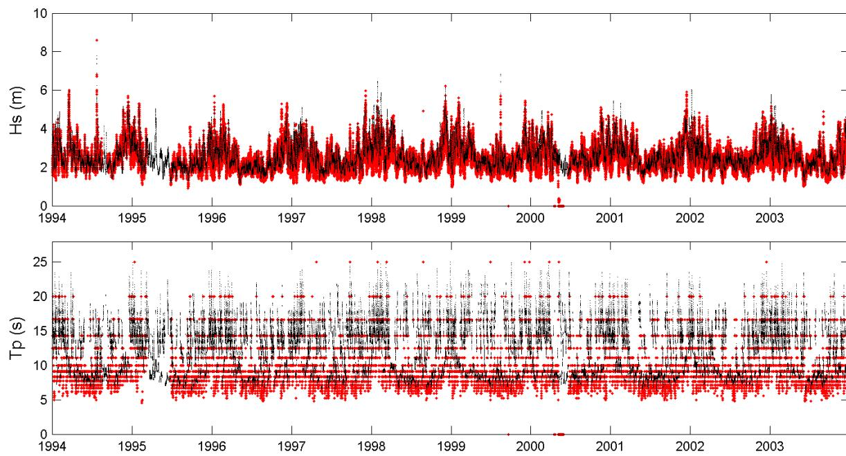
Figure 17- Comparison of recorded (red) and hindcast (black) wave parameters at buoy #51002 from 1994 to 2003.
