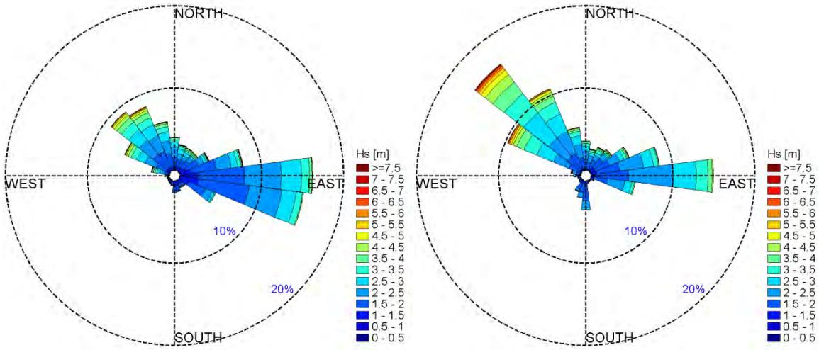
Figure 42- Rose plots of recorded (left) and hindcast (right) significant wave heights at buoy #51101.
