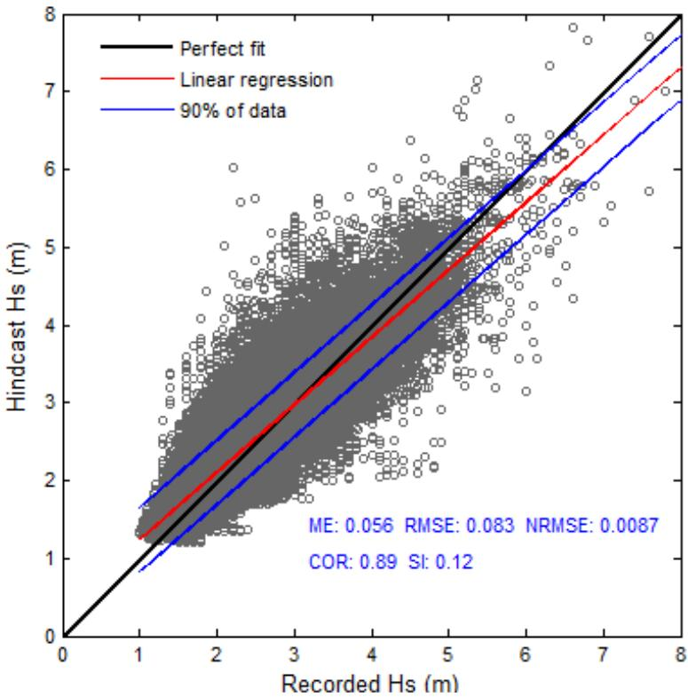
Figure 27- Scatter plot of recorded and hindcast significant wave heights at buoy #51004.
