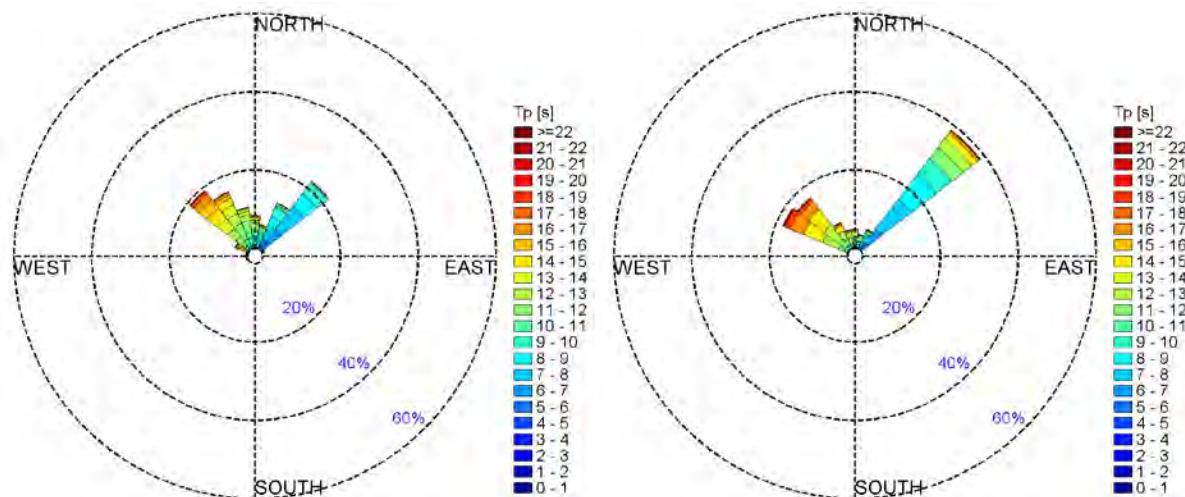
Figure 69- Rose plots of recorded (left) and hindcast (right) peak periods at the Waimea buoy.
