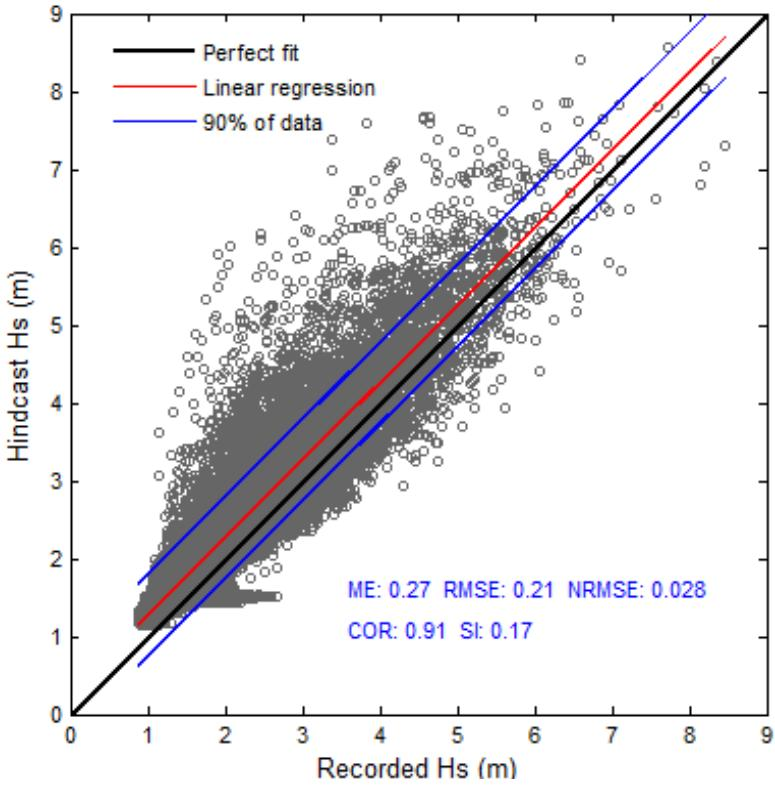
Figure 29- Scatter plot of recorded and hindcast significant wave heights at buoy #51101.
