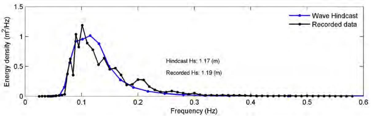
Figure 83- One-dimensional spectra estimated from WETS Waverider records and hindcast model at 4:00 PM May 5, 2013.
