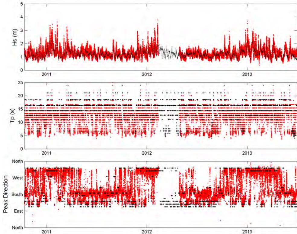
Figure 45 - Comparison of recorded (red) and hindcast (black) wave parameters at the Barbers Point buoy.
