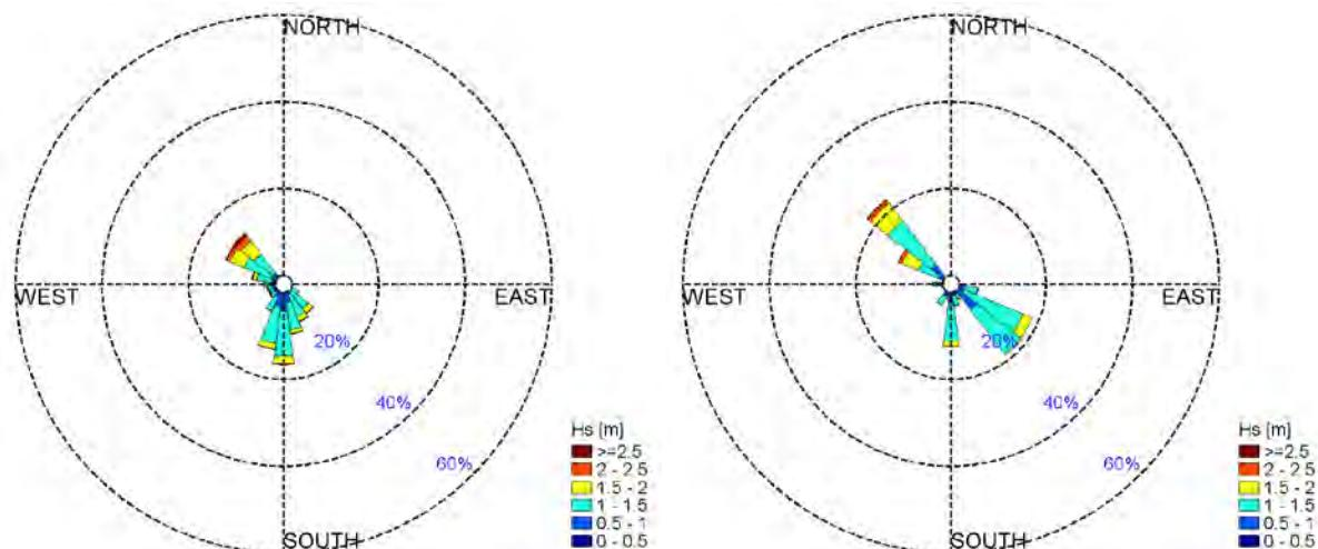
Figure 70- Rose plots of recorded (left) and hindcast (right) significant wave heights at the Barbers Point buoy.
