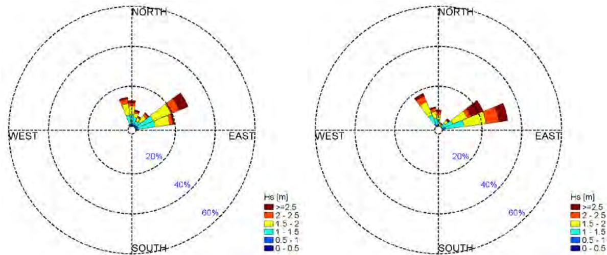
Figure 74- Rose plots of recorded (left) and hindcast (right) significant wave heights at the WETS buoy.
