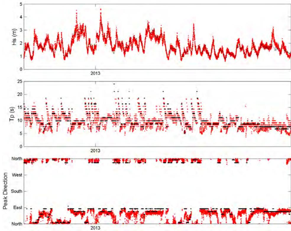
Figure 47- Comparison of recorded (red) and hindcast (black) wave parameters at the WETS buoy.
