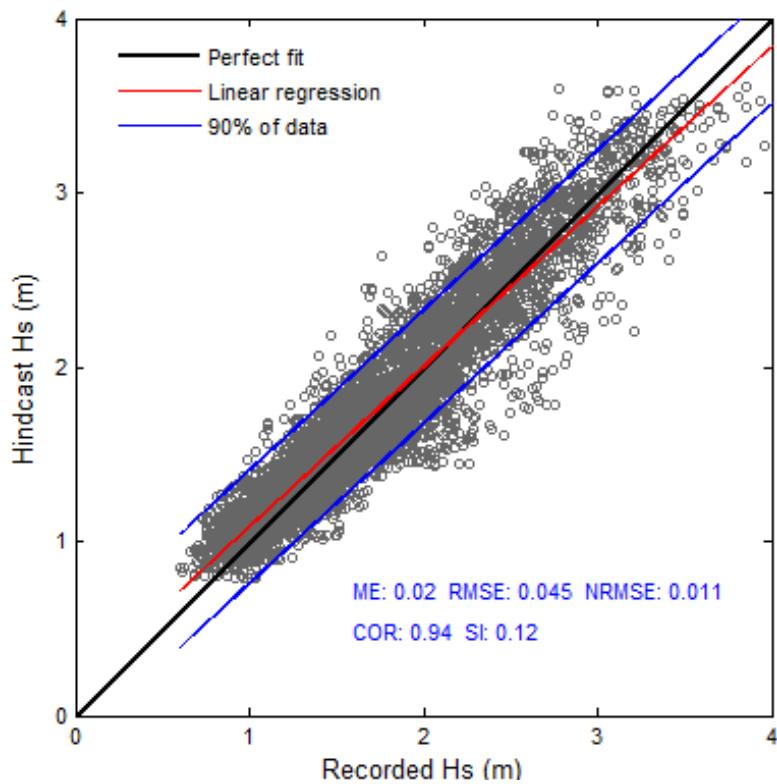
Figure 51- Scatter plot of recorded and hindcast significant wave heights at the WETS buoy.
