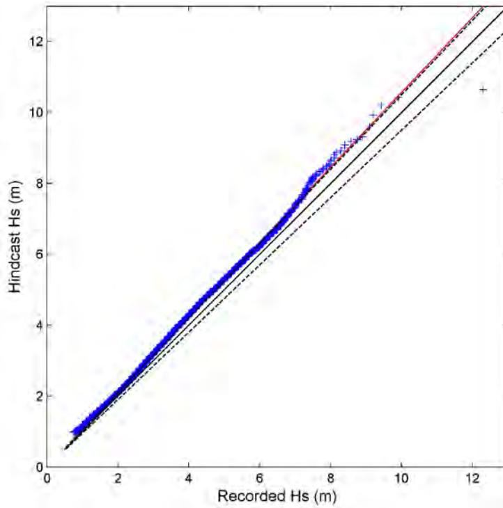
Figure 30- Quantile-quantile plot of recorded and hindcast significant wave heights at buoy #51001. Blue crosses represent data pair at 0.002 percentile increment, black line denotes perfect match, black dash lines delineate the  $\pm 5\%$  error bounds, and red line is the linear regression.
