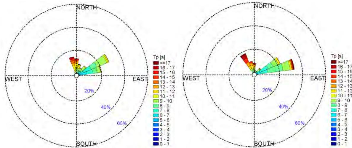
Figure 75- Rose plots of recorded (left) and hindcast (right) peak periods at the WETS buoy.
