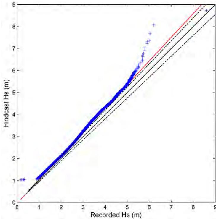
Figure 32- Quantile-quantile plot of recorded and hindcast significant wave heights at buoy #51002. Blue crosses represent data pair at 0.002 percentile increment, black line denotes perfect match, black dash lines delineate the  $\pm 5\%$  error bounds, and red line is the linear regression.
