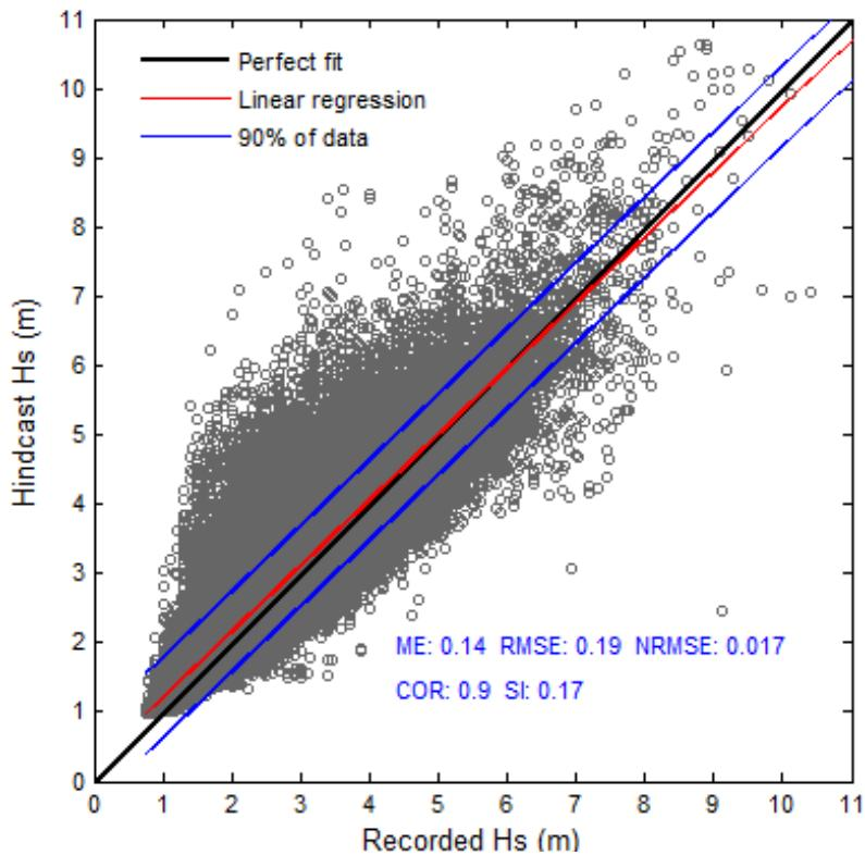
Figure 24- Scatter plot of recorded and hindcast significant wave heights at buoy #51001.
