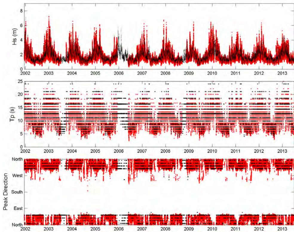
Figure 44- Comparison of recorded (red) and hindcast (black) wave parameters at the Waimea buoy.
