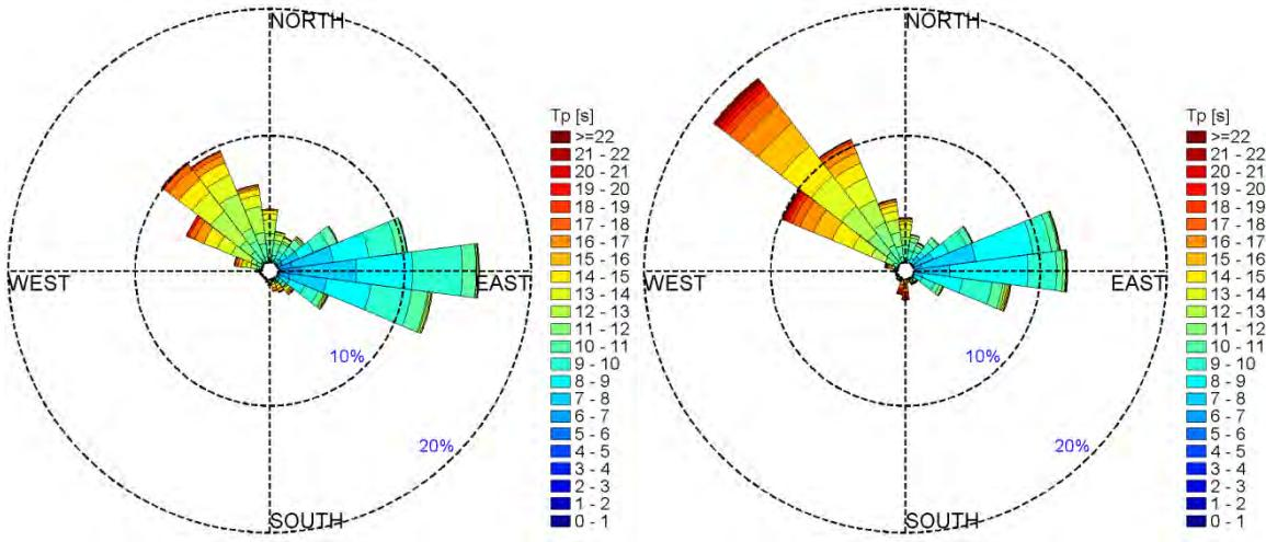
Figure 41- Rose plots of recorded (left) and hindcast (right) peak periods at buoy #51100.
