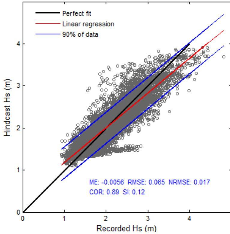
Figure 63- Scatter plot of recorded and hindcast significant wave heights at the Hilo buoy.
