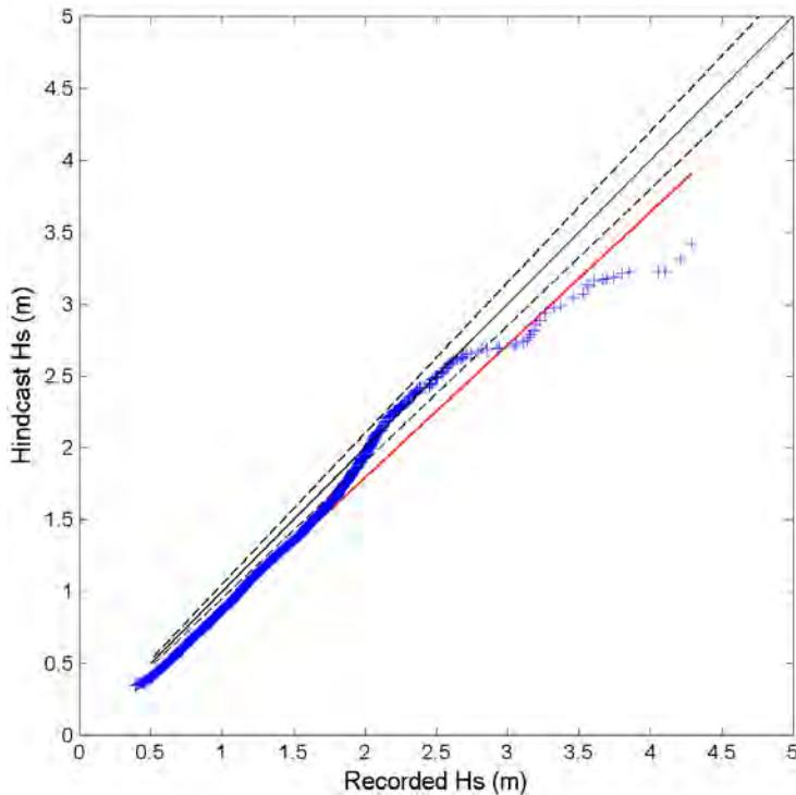
Figure 66- Quantile-quantile plot of recorded and hindcast significant wave heights at the Kaumalapau buoy. Blue crosses represent data pair at 0.002 percentile increment, black line denotes perfect match, black dash lines delineate the  $\pm 5\%$  error bounds, and red line is the linear regression.
