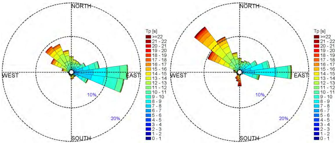
Figure 43- Rose plots of recorded (left) and hindcast (right) peak periods at buoy # 51101.
