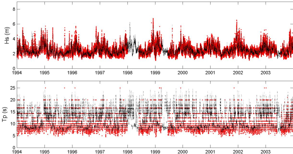
Figure 20- Comparison of recorded (red) and hindcast (black) wave parameters at buoy #51004 from 1994 to 2003.
