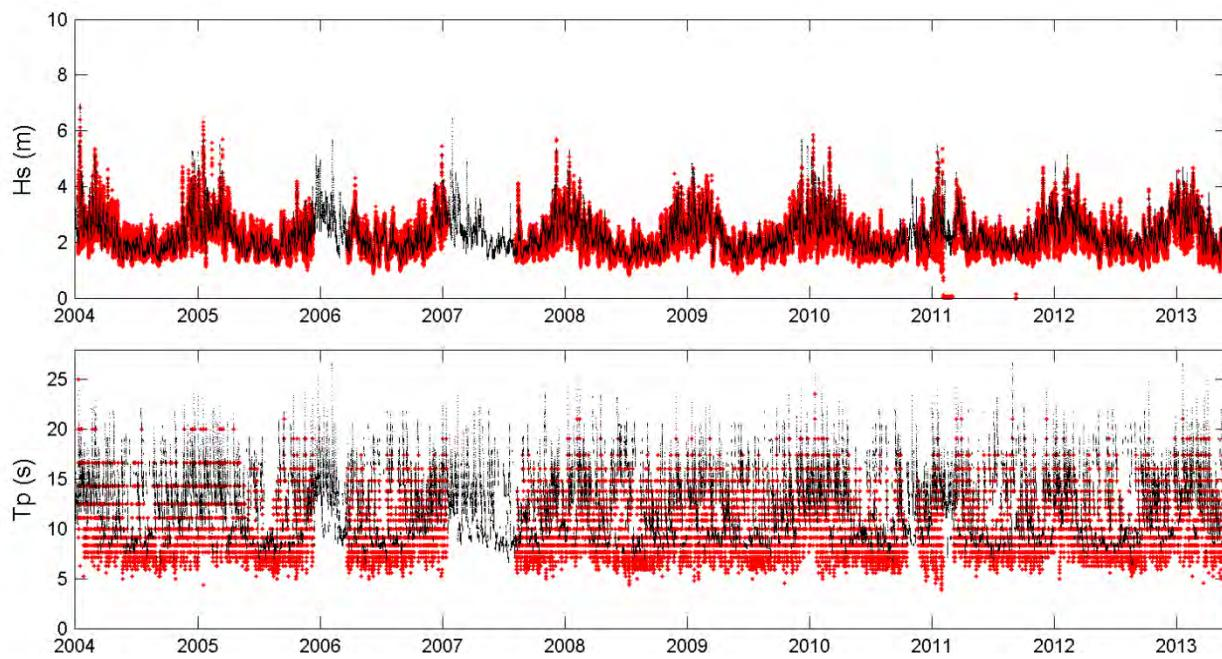
Figure 15- Comparison of recorded (red) and hindcast (black) wave parameters at buoy #51003 from 2004 to 2013.
