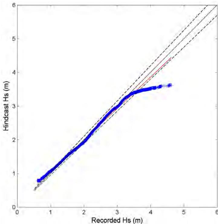
Figure 55- Quantile-quantile plot of recorded and hindcast significant wave heights at the WETS buoy. Blue crosses represent data pair at 0.002 percentile increment, black line denotes perfect match, black dash lines delineate the  $\pm 5\%$  error bounds, and red line is the linear regression.
