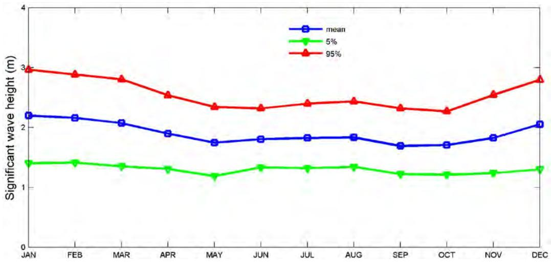
Figure 108– Monthly statistics of significant wave height at site South Point.
