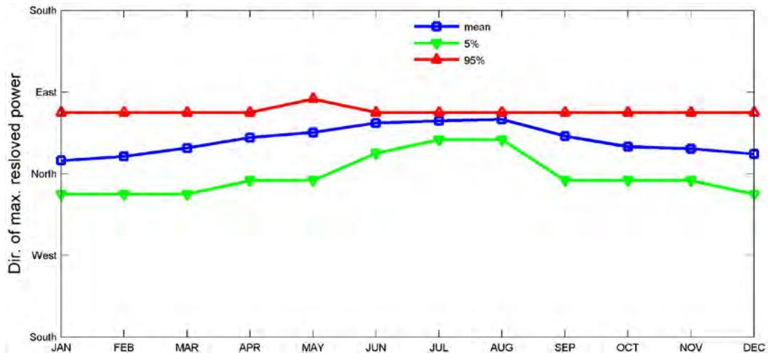
Figure 90– Monthly statistics of direction of maximum directionally resolved wave power at WETS.
