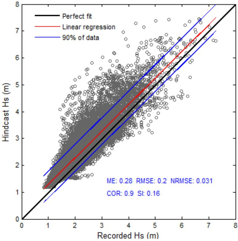
Figure 28- Scatter plot of recorded and hindcast significant wave heights at buoy #51100.
