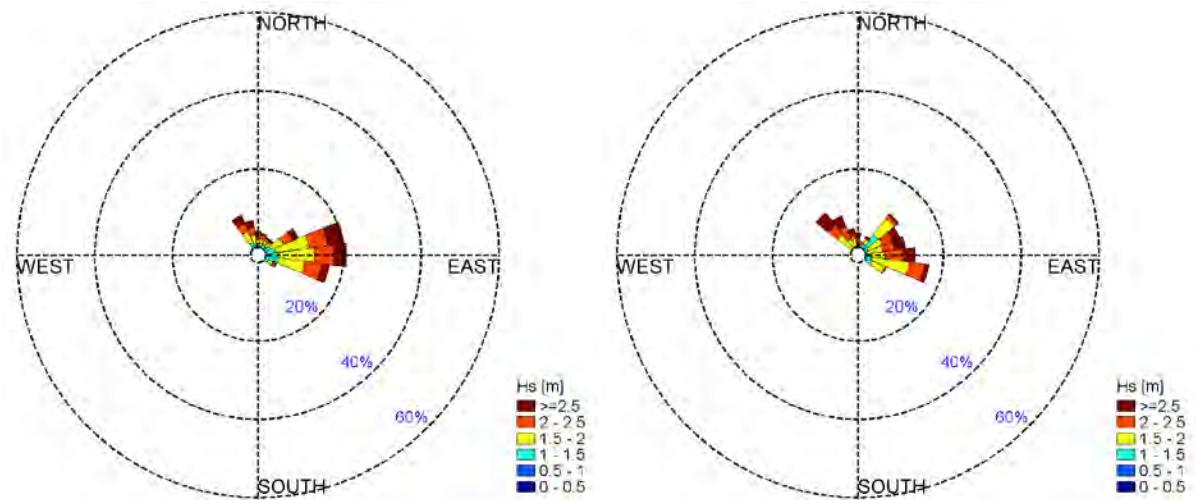
Figure 80- Rose plots of recorded (left) and hindcast (right) significant wave heights at the Hilo buoy.
