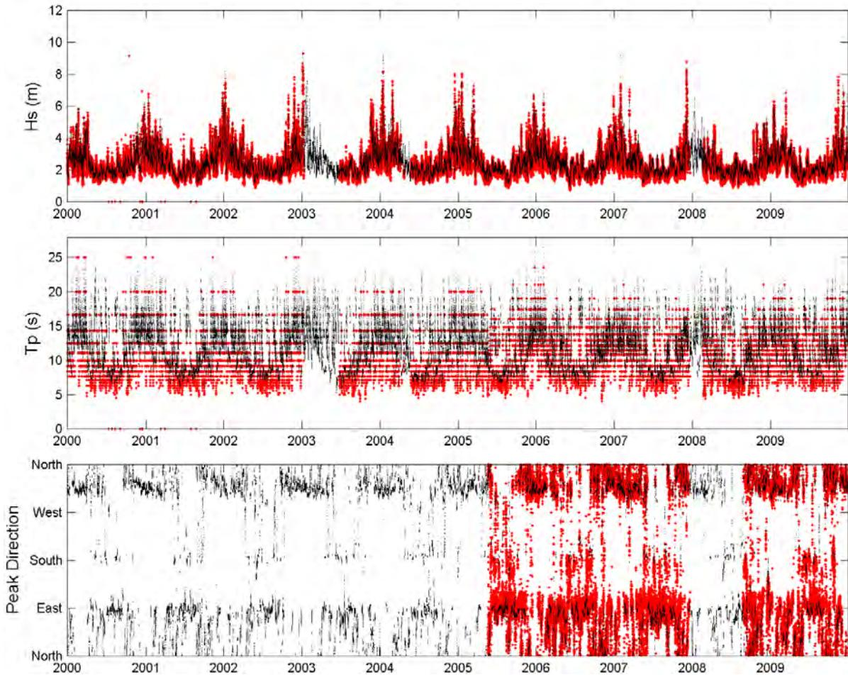
Figure 12- Comparison of recorded (red) and hindcast (black) wave parameters at buoy #51001 from 2000 to 2009.
