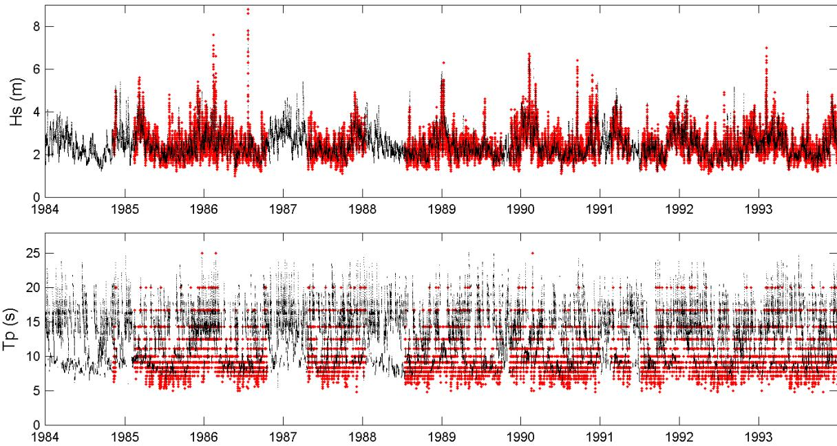
Figure 19- Comparison of recorded (red) and hindcast (black) wave parameters at buoy #51004 from 1984 to 1993.
