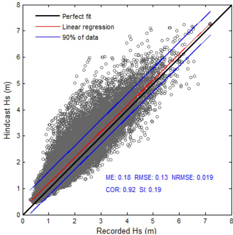
Figure 48- Scatter plot of recorded and hindcast significant wave heights at the Waimea buoy.
