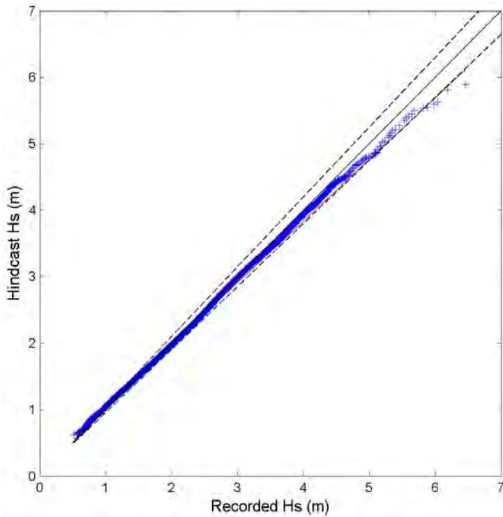
Figure 54- Quantile-quantile plot of recorded and hindcast significant wave heights at Mokapu buoy. Blue crosses represent data pair at 0.002 percentile increment, black line denotes perfect match, black dash lines delineate the  $\pm 5\%$  error bounds, and red line is the linear regression.
