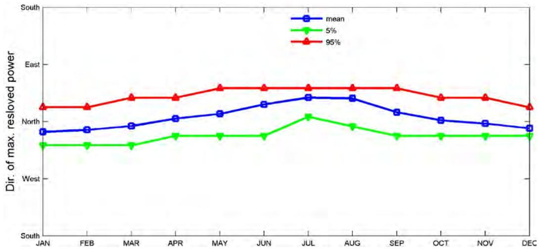
Figure 121– Monthly statistics of direction of maximum directionally resolved wave power at site Kilauea.
