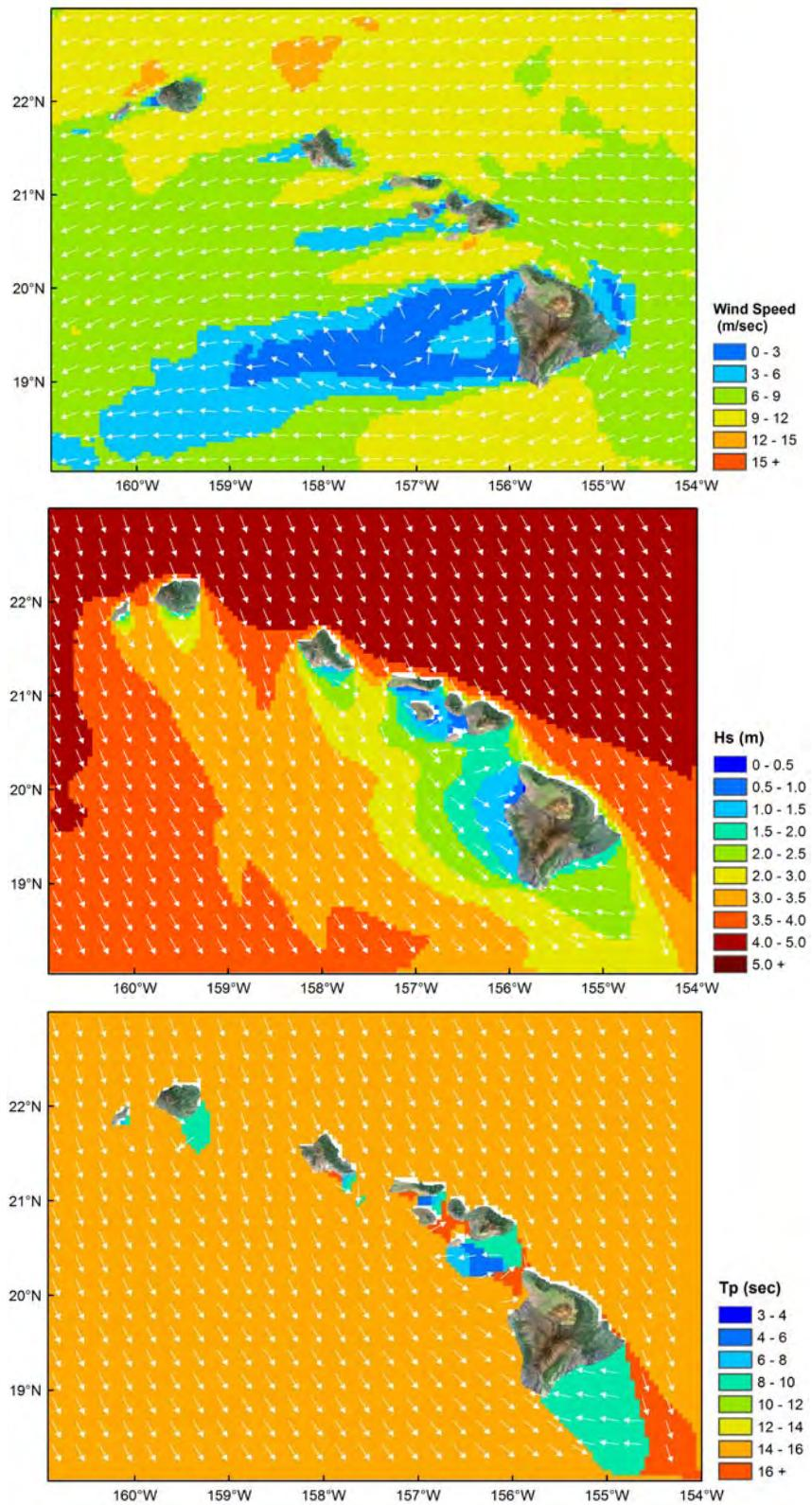
Figure 8- Wind velocity, significant wave height, and peak period during a northwest swell event at 9:00 AM March 16, 2010 UTC.
