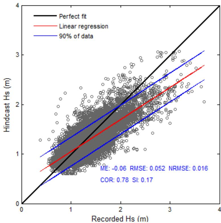
Figure 49- Scatter plot of recorded and hindcast significant wave heights at the Barbers Point buoy.
