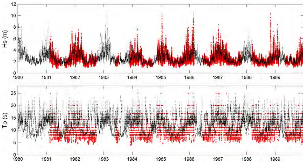
Figure 10- Comparison of recorded (red) and hindcast (black) wave parameters at buoy #51001 from 1980 to 1989.
