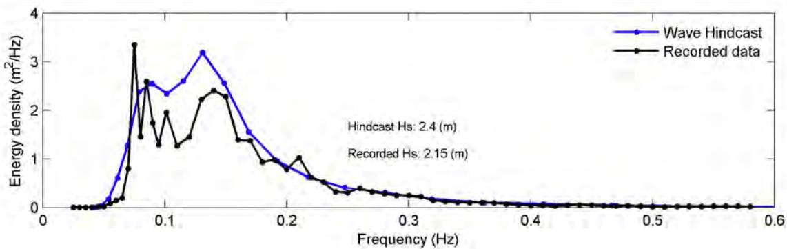
Figure 85- One-dimensional spectra estimated from WETS Waverider records and hindcast model at 1:00 AM January 4, 2013.
