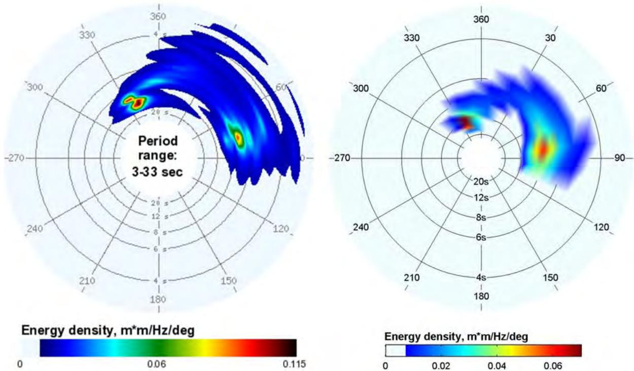
Figure 84- Two-dimensional spectra estimated from WETS Waverider records (left) and hindcast model (right) at 1:00 AM January 4, 2013.
