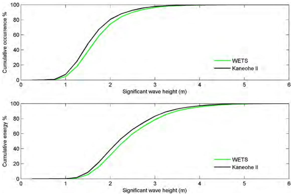
Figure 102– Cumulative distributions of significant wave height (upper) and the associated wave energy (lower) in terms of the percentage total at WETS and site Kaneohe II.
