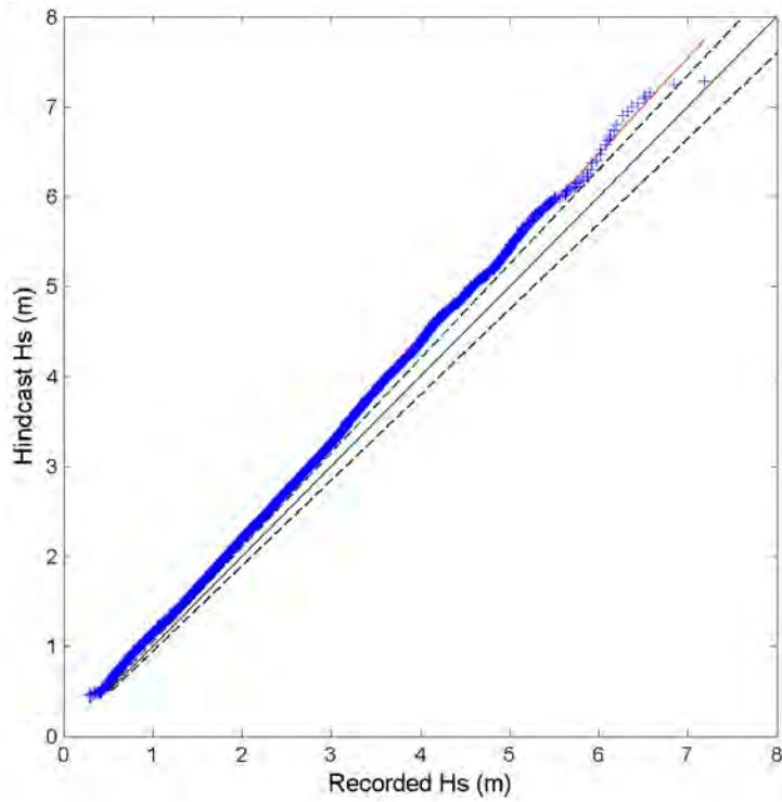
Figure 52- Quantile-quantile plot of recorded and hindcast significant wave heights at the Waimea buoy. Blue crosses represent data pair at 0.002 percentile increment, black line denotes perfect match, black dash lines delineate the  $\pm 5\%$  error bounds, and red line is the linear regression.
