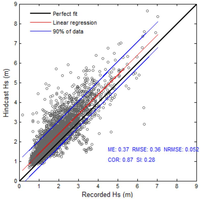
Figure 60- Scatter plot of recorded and hindcast significant wave heights at the Barking Sands buoy.
