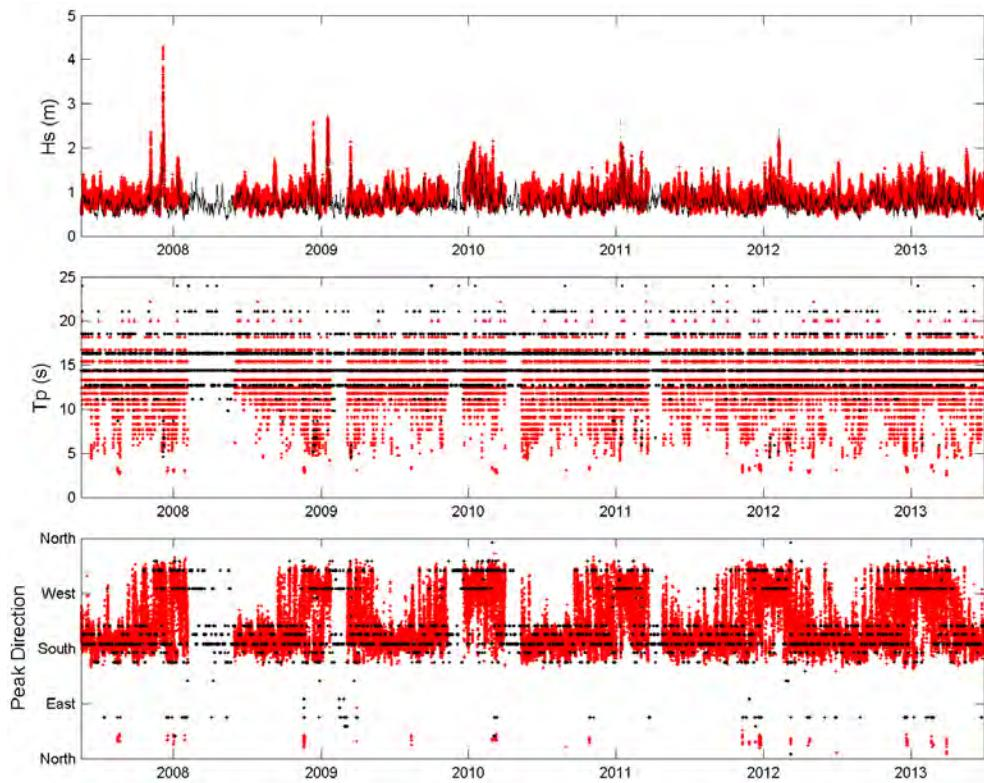
Figure 58- Comparison of recorded (red) and hindcast (black) wave parameters at the Kaumalapau buoy.
