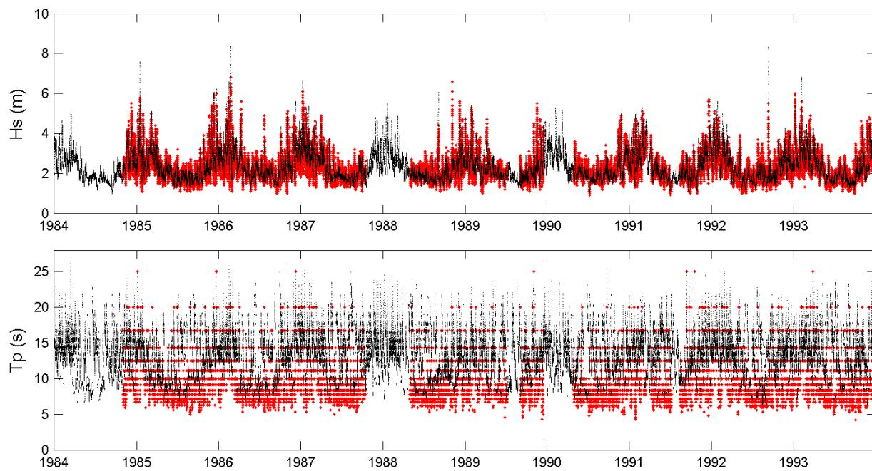
Figure 13- Comparison of recorded (red) and hindcast (black) wave parameters at buoy #51003 from 1984 to 1993.
