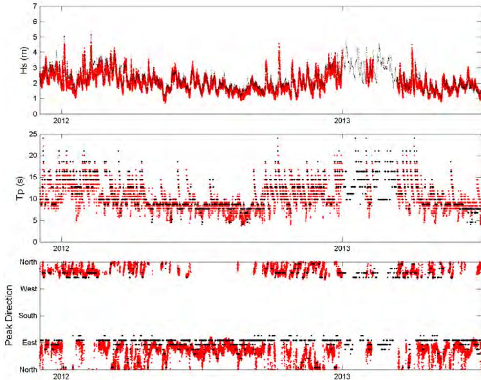
Figure 57- Comparison of recorded (red) and hindcast (black) wave parameters at the Pauwela buoy.
