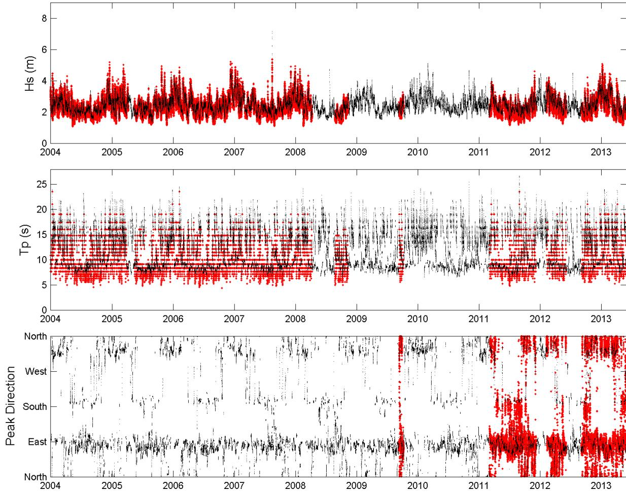
Figure 21- Comparison of recorded (red) and hindcast (black) wave parameters at buoy #51004 from 2004 to 2013.
