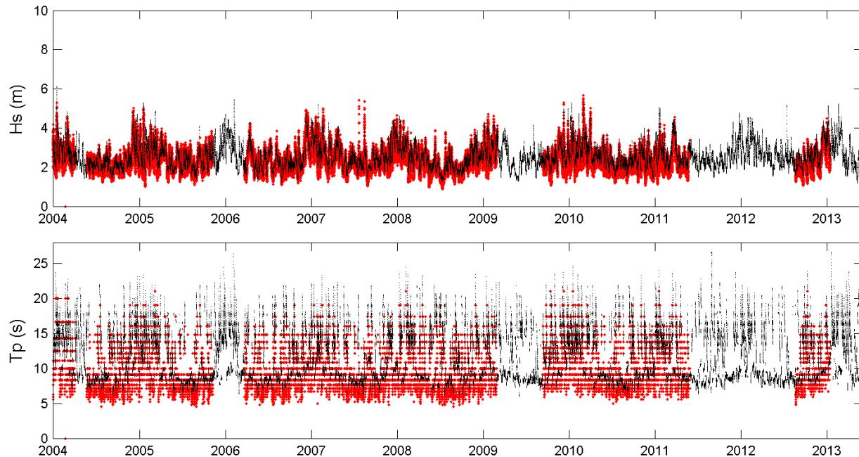
Figure 18- Comparison of recorded (red) and hindcast (black) wave parameters at buoy #51002 from 2004 to 2013.
