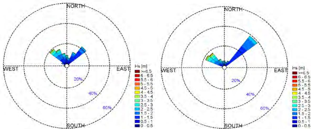
Figure 68- Rose plots of recorded (left) and hindcast (right) significant wave heights at the Waimea buoy.
