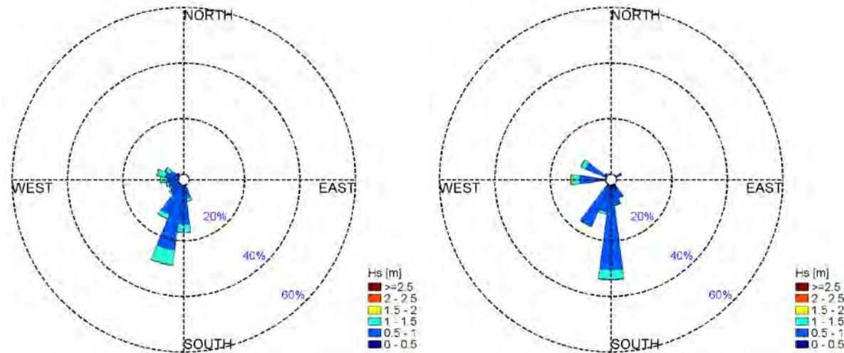
Figure 78- Rose plots of recorded (left) and hindcast (right) significant wave heights at the Kaumalapau buoy.
