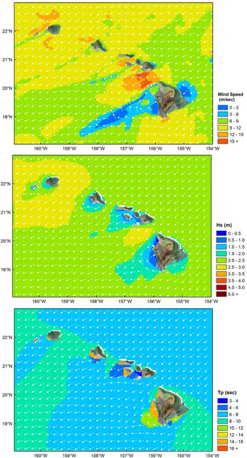
Figure 6- Wind velocity, significant wave height, and peak period during a trade wind event at 3:00 AM June 28, 2012UTC.
