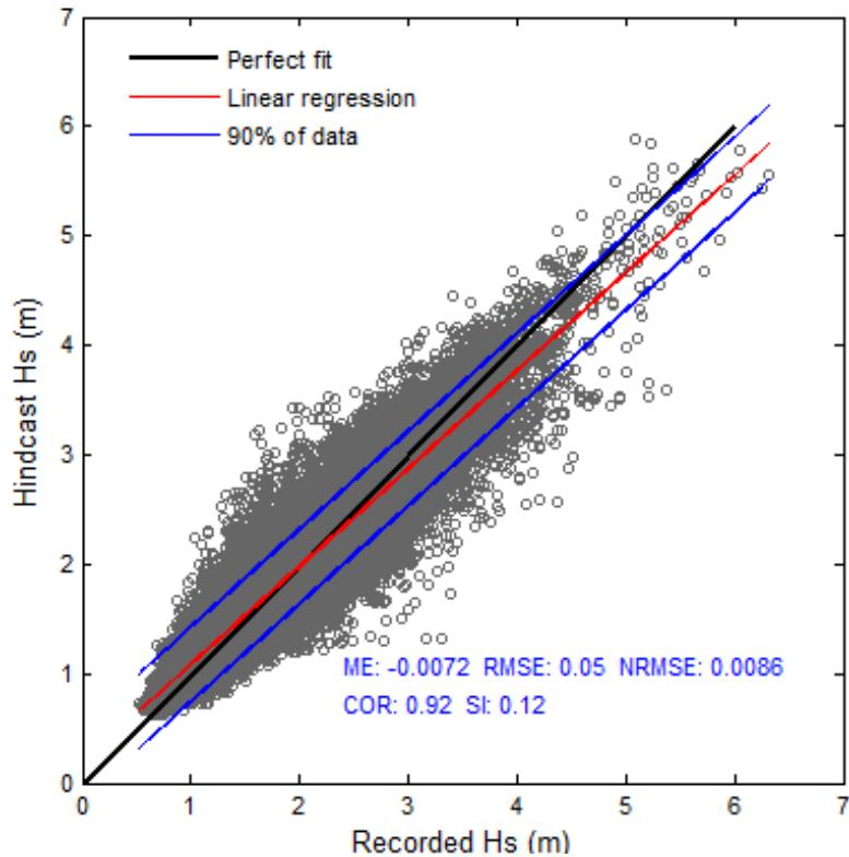
Figure 50- Scatter plot of recorded and hindcast significant wave heights at the Mokapu buoy.
