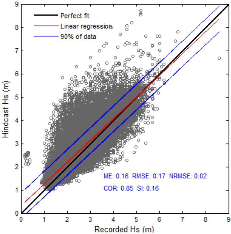
Figure 26- Scatter plot of recorded and hindcast significant wave heights at buoy #51002.
