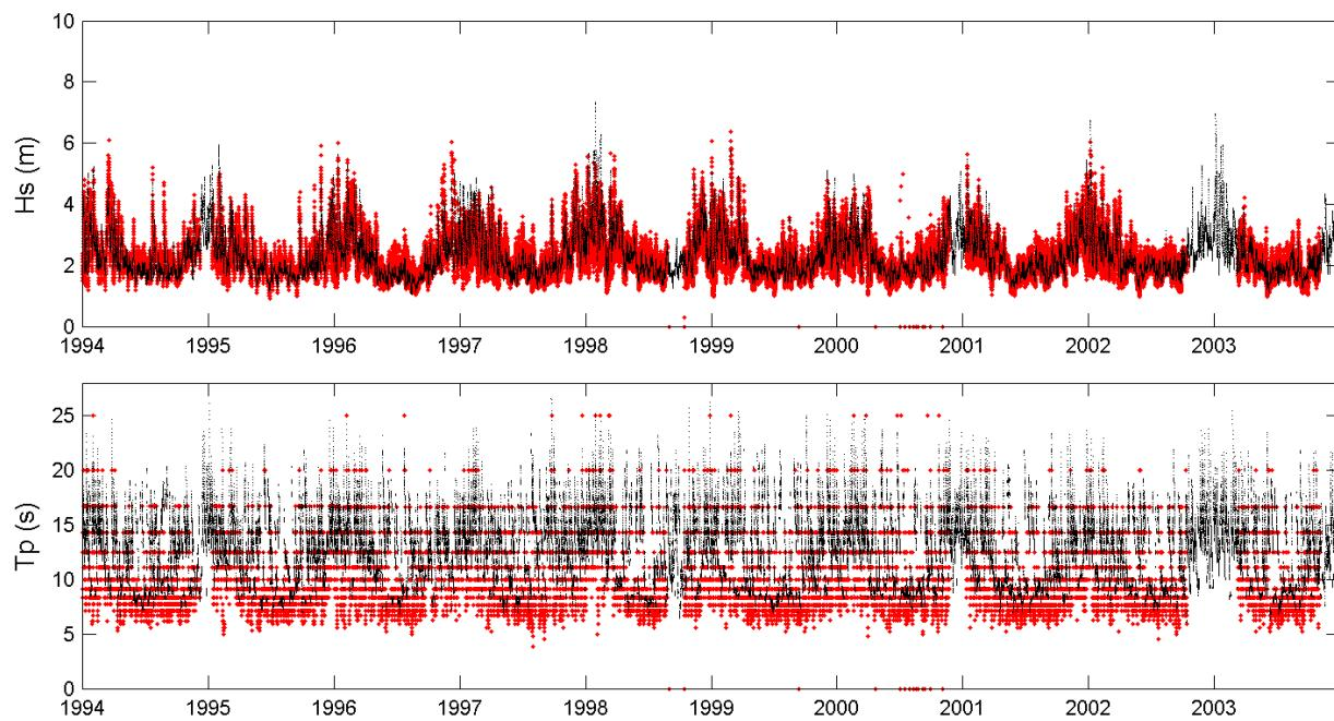
Figure 14- Comparison of recorded (red) and hindcast (black) wave parameters at buoy #51003 from 1994 to 2003.
