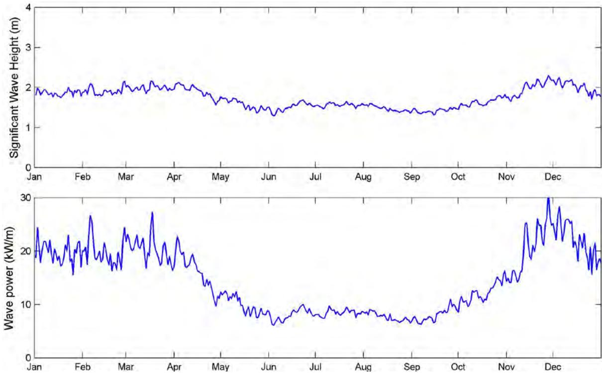
Figure A1– Average daily significant wave height and wave power at WETS.
