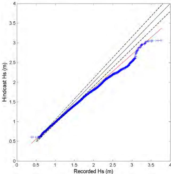
Figure 53- Quantile-quantile plot of recorded and hindcast significant wave heights at the Barbers Point buoy. Blue crosses represent data pair at 0.002 percentile increment, black line denotes perfect match, black dash lines delineate the  $\pm 5\%$  error bounds, and red line is the linear regression.
