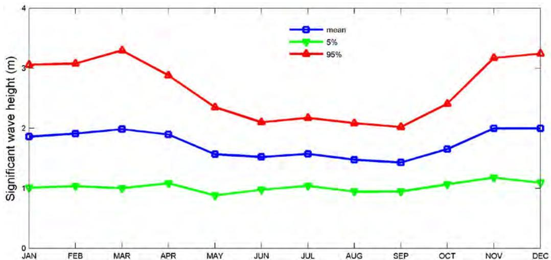
Figure 86– Monthly statistics of significant wave height at WETS.
