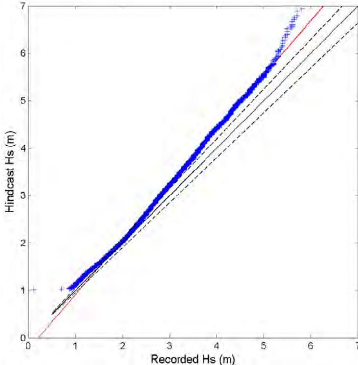
Figure 31- Quantile-quantile plot of recorded and hindcast significant wave heights at buoy #51003. Blue crosses represent data pair at 0.002 percentile increment, black line denotes perfect match, black dash lines delineate the  $\pm 5\%$  error bounds, and red line is the linear regression.
