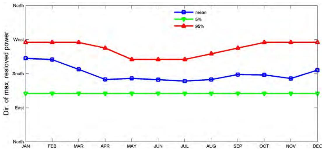
Figure 124– Monthly statistics of direction of maximum directionally resolved wave power at site South Point.
