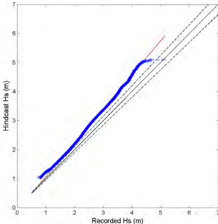
Figure 65- Quantile-quantile plot of recorded and hindcast significant wave heights at the Pauwela buoy. Blue crosses represent data pair at 0.002 percentile increment, black line denotes perfect match, black dash lines delineate the  $\pm 5\%$  error bounds, and red line is the linear regression.
