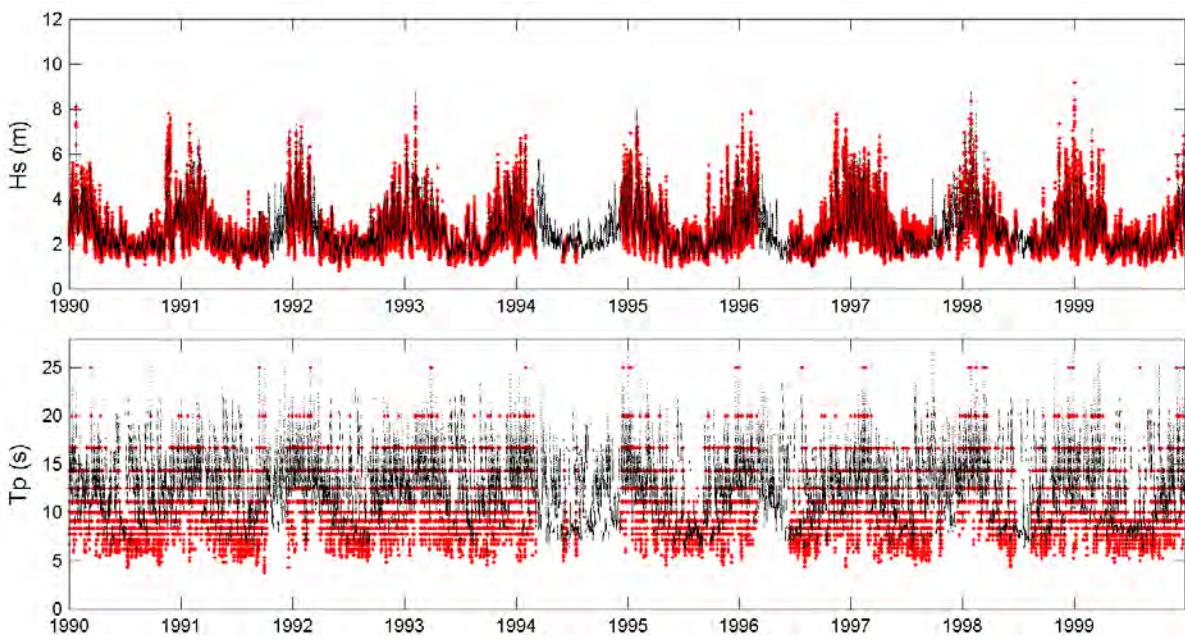
Figure 11- Comparison of recorded (red) and hindcast (black) wave parameters at buoy #51001 from 1990 to 1999.
