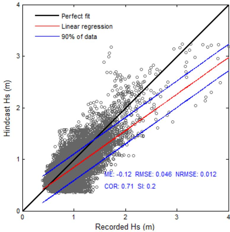
Figure 62- Scatter plot of recorded and hindcast significant wave heights at the Kaumalapau buoy.
