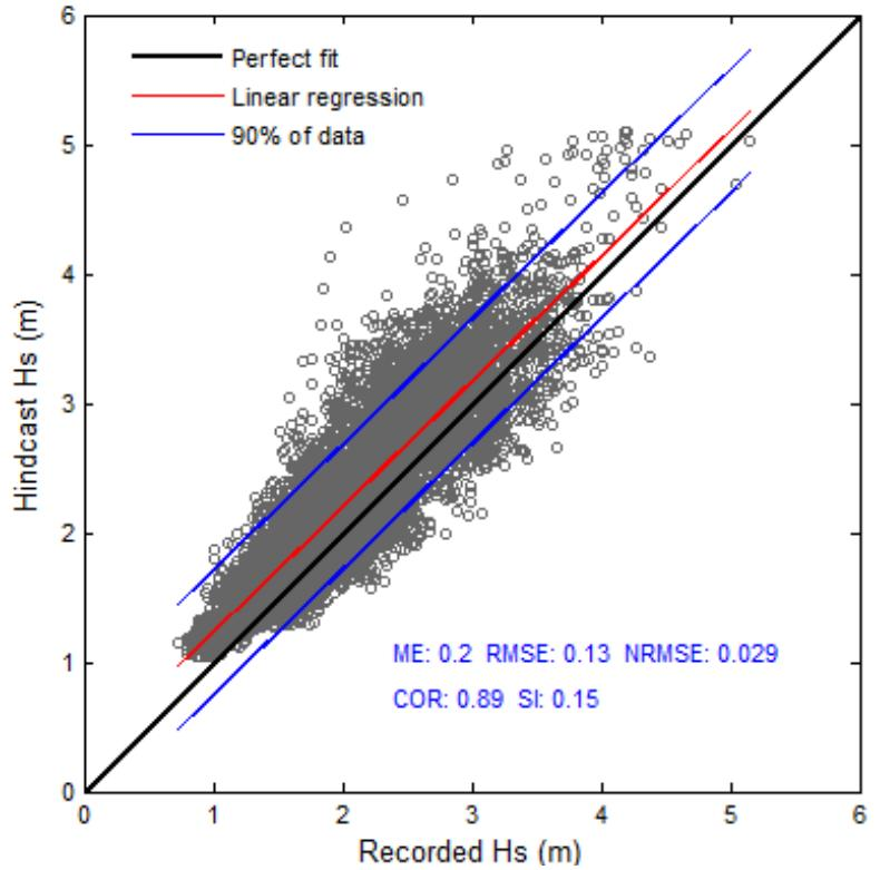
Figure 61- Scatter plot of recorded and hindcast significant wave heights at the Pauwela buoy.
