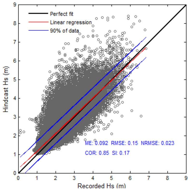
Figure 25- Scatter plot of recorded and hindcast significant wave heights at buoy #51003.
