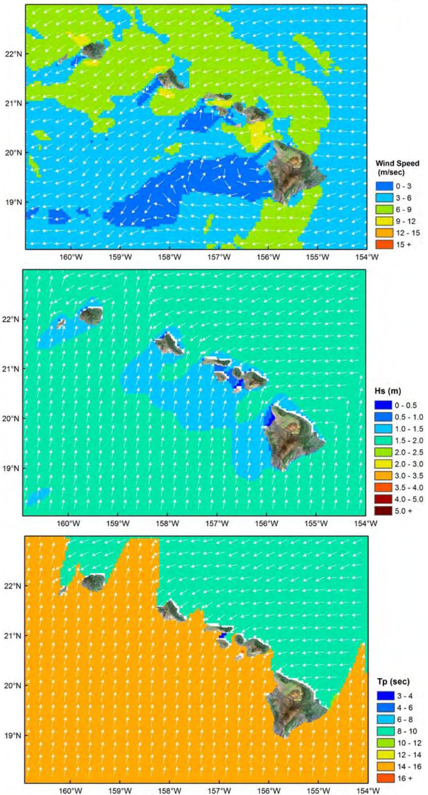
Figure 7- Wind velocity, significant wave height and peak period during a south swell event at 0:00 AM August 30, 2007 UTC.
