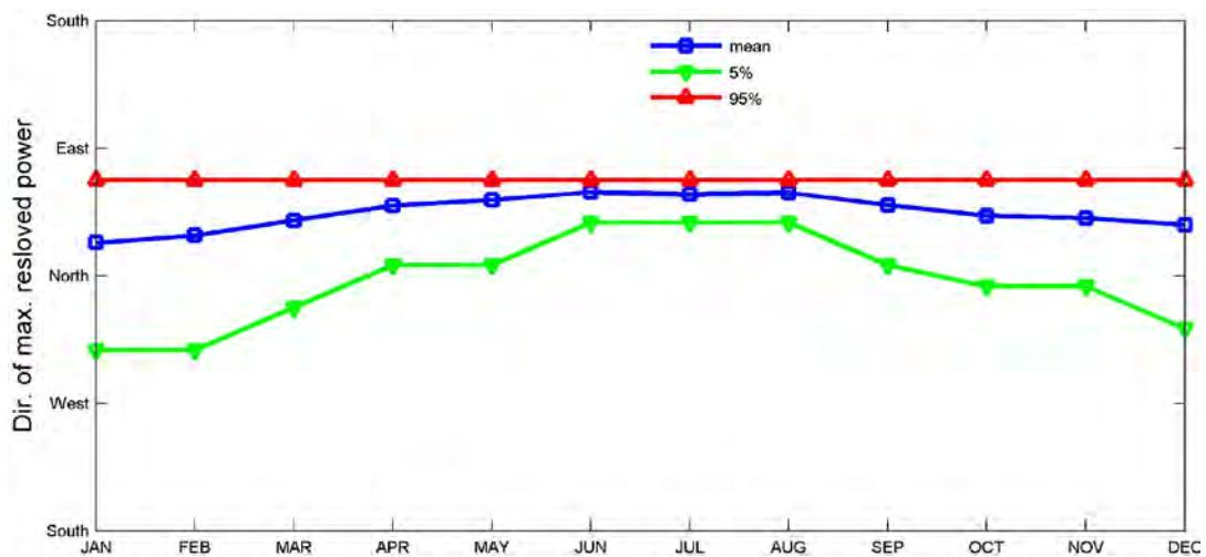
Figure 123– Monthly statistics of direction of maximum directionally resolved wave power at site Upolu.
