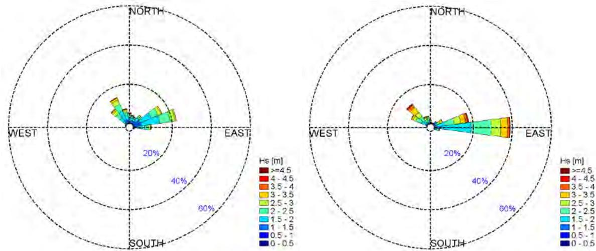
Figure 76- Rose plots of recorded (left) and hindcast (right) significant wave heights at the Pauwela buoy.
