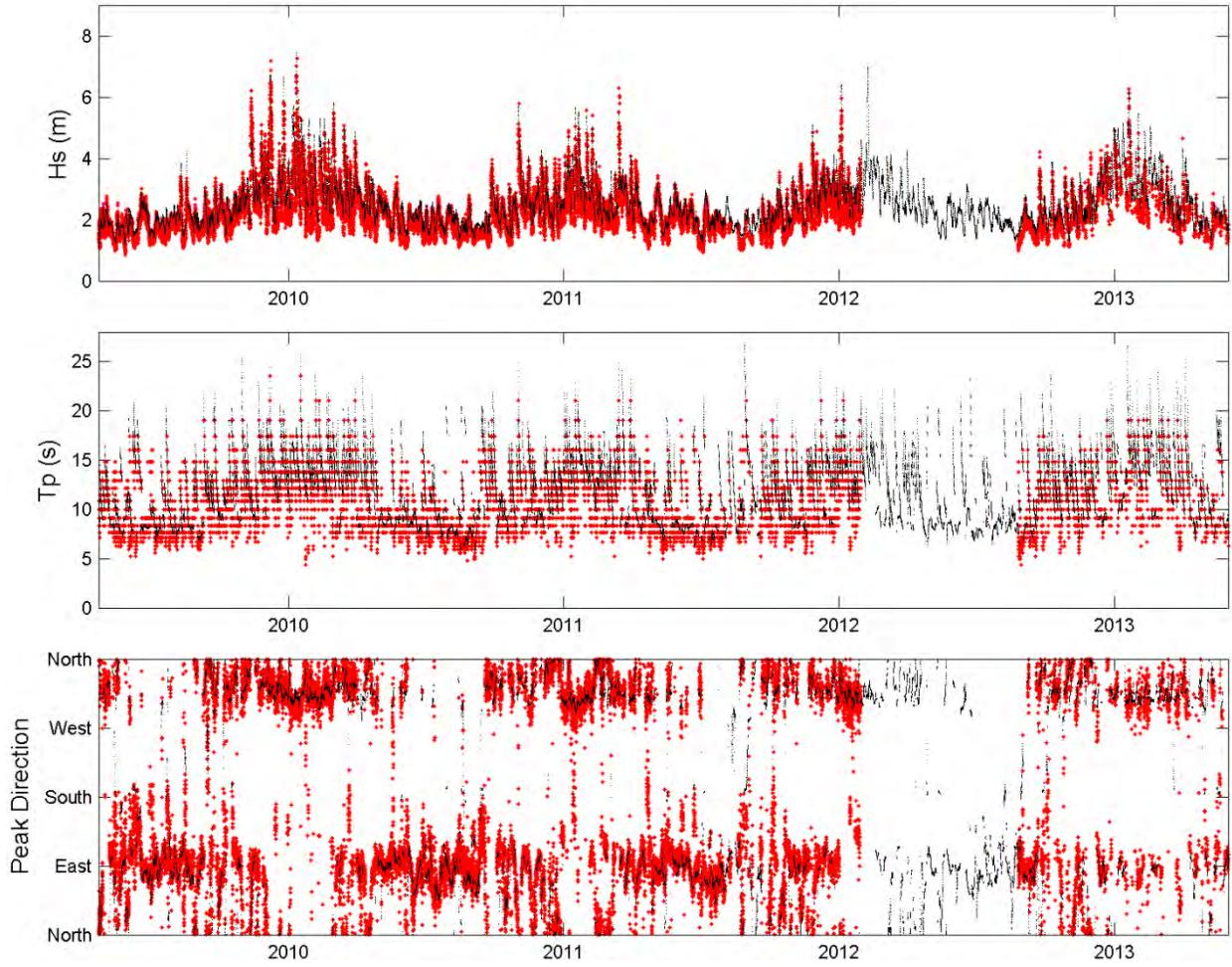
Figure 22- Comparison of recorded (red) and hindcast (black) wave parameters at buoy #51100 from 2009 to 2013.
